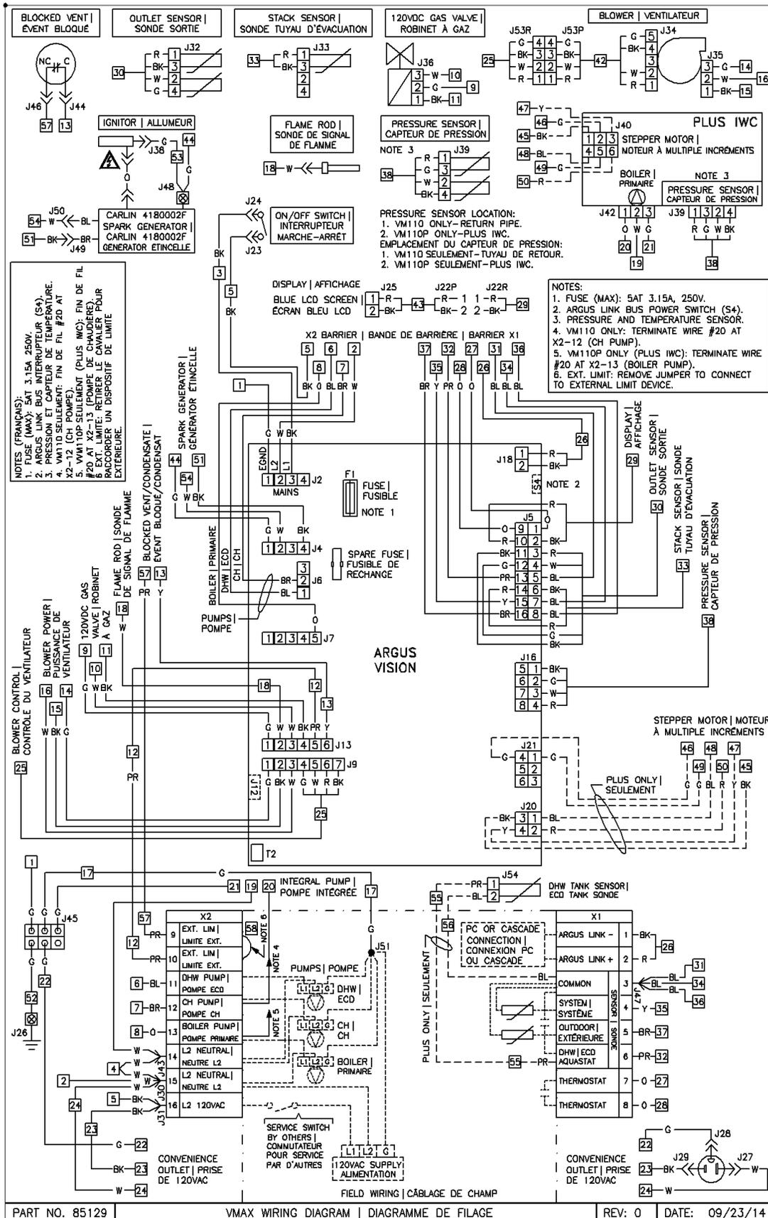
Figure 14-2 Vmax Ladder-Logic Diagram
