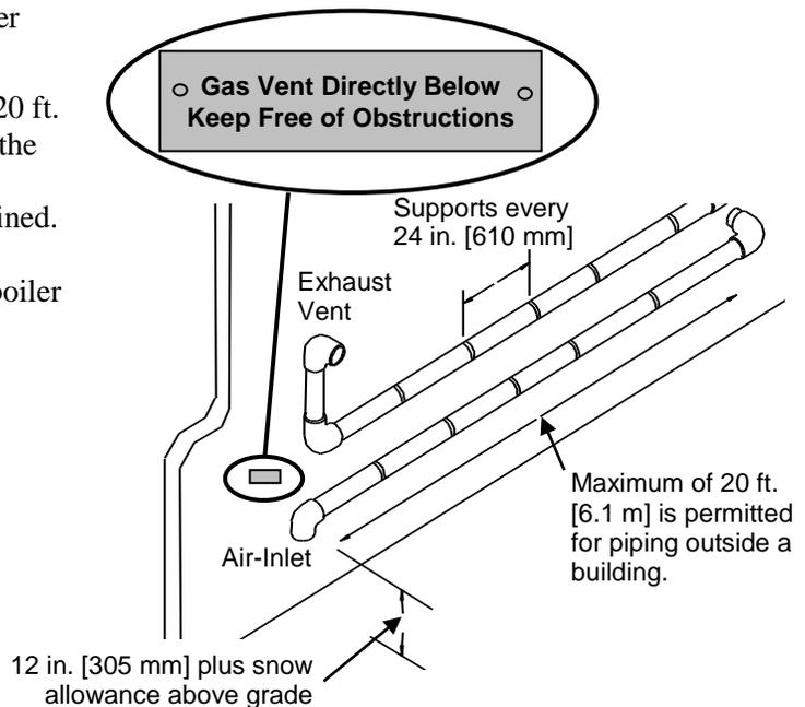
**Figure 4-10 Existing Chimney Chase Way**
