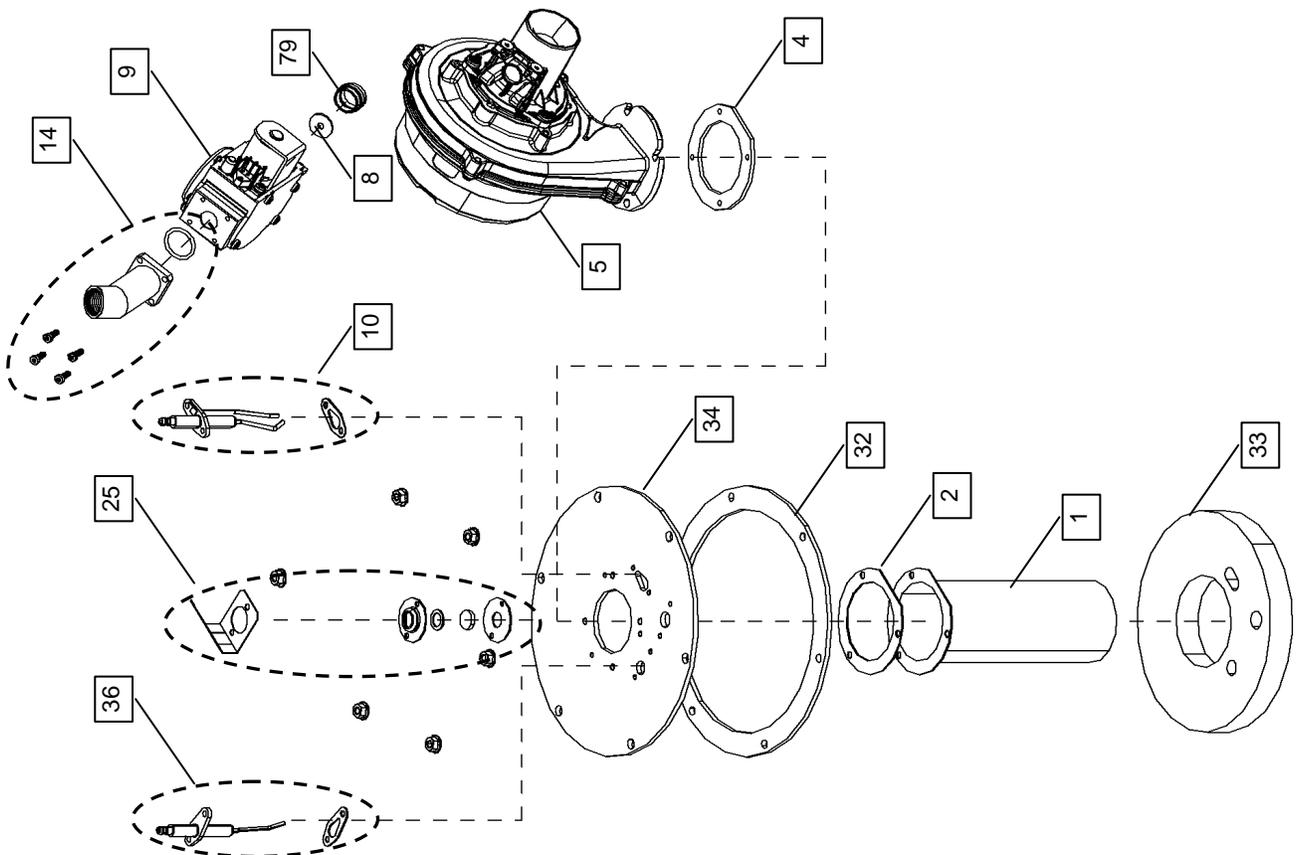
Figure 19-1(d) Vmax Cabinet & Controls (VM110P illustrated)
