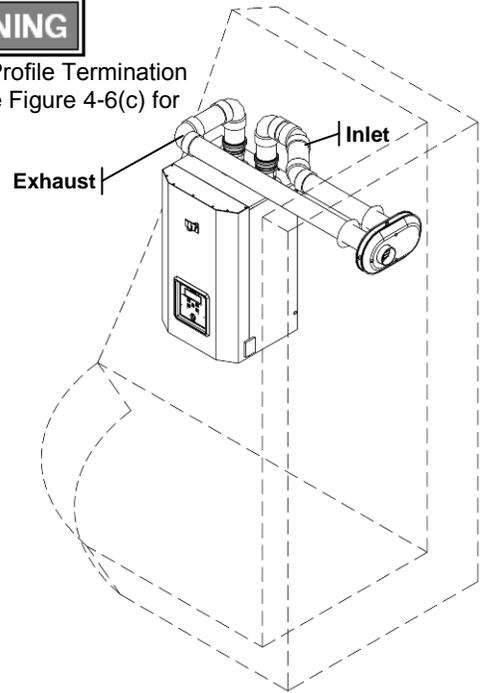
Figure 4-4(c) Concentric Termination (Sidewall)
