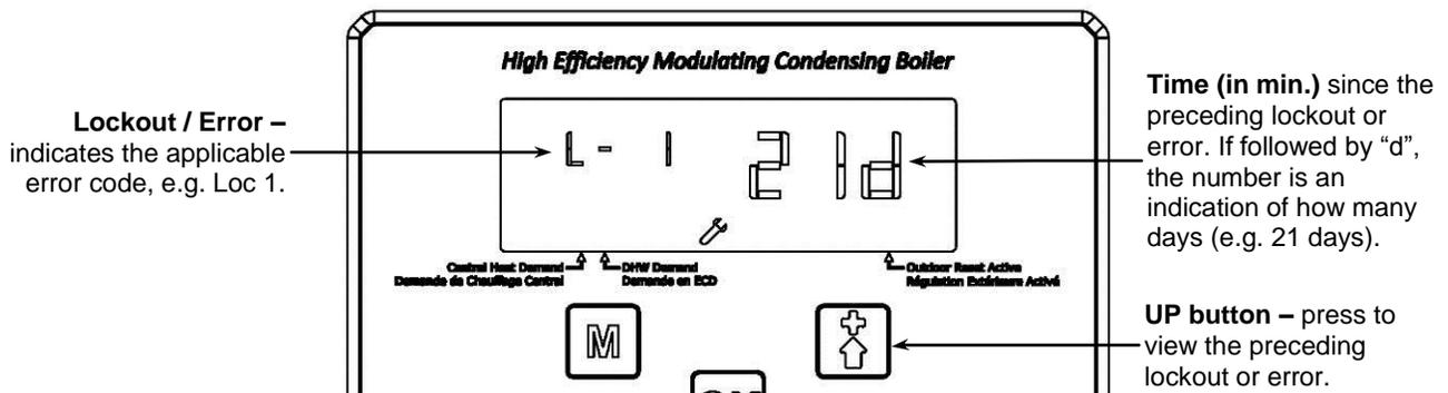
Figure 17-5(c) Lockout and Error History Navigation (End)
