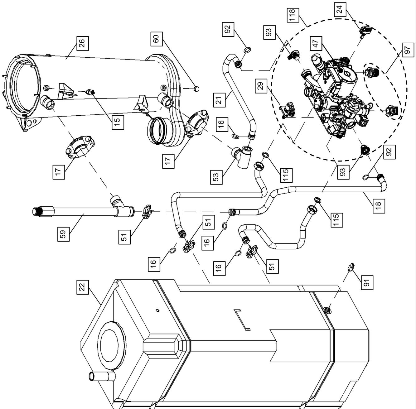
Figure 19-1(b) VM110 Heat Exchanger, Water Piping & Sensors
