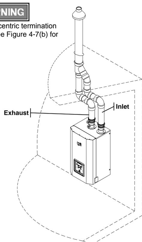
Sidewall Termination Details – Direct Vent Installation
