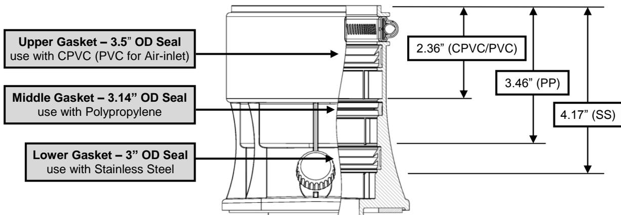
Figure 4-2 (b) Universal Exhaust-vent & Air-inlet Appliance Adapter
