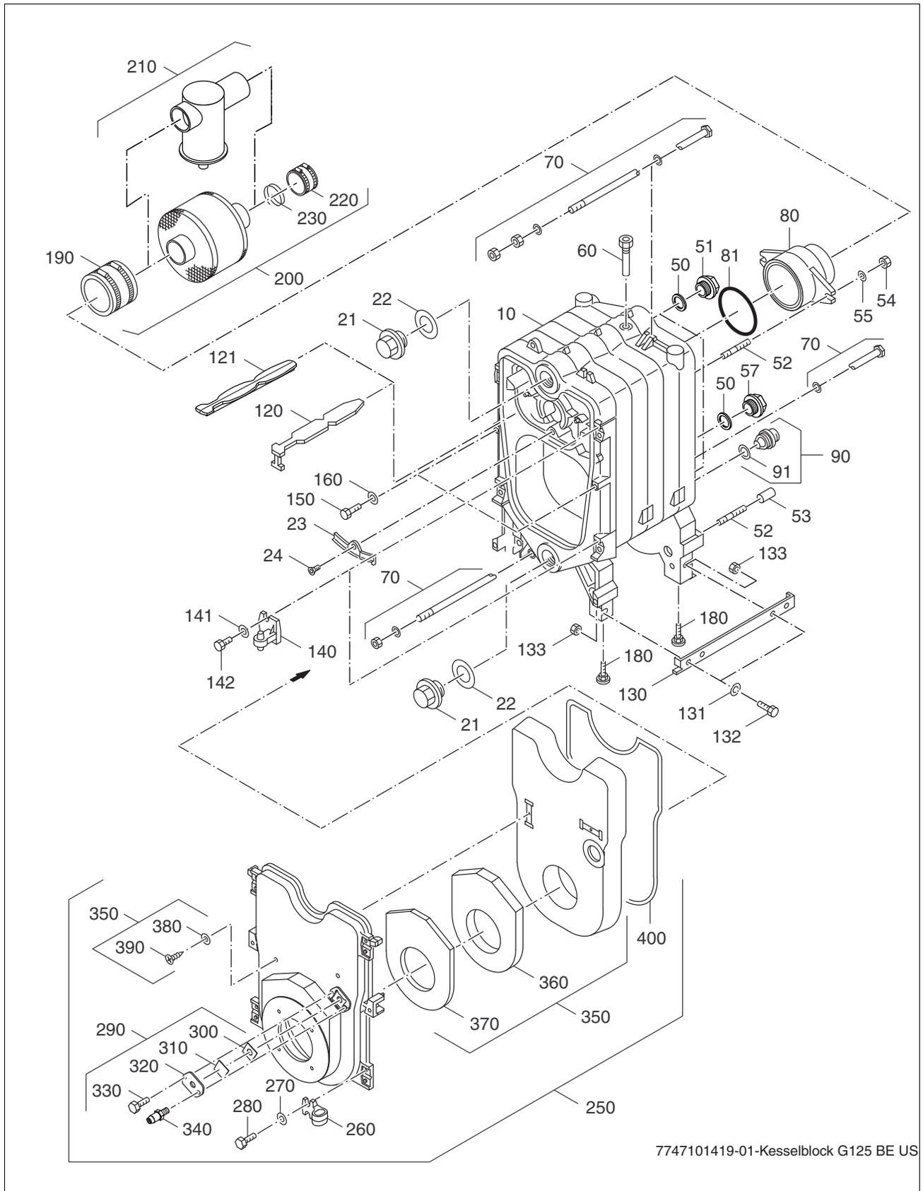
Fig. 60 Boiler block and burner door
