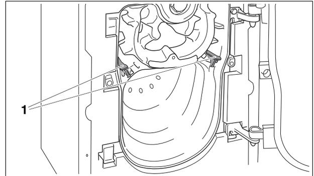
Fig. 50 Opening of burner door
