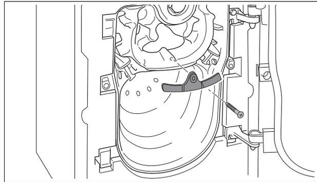
Fig.46 Removal of flue blocking plate
