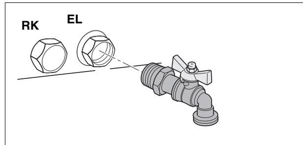
Fig. 24 Boiler Drain installation
