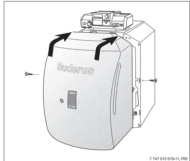
Fig.47 Installation of burner cover
