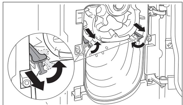
Fig.43 Adjusting the flue baffles
