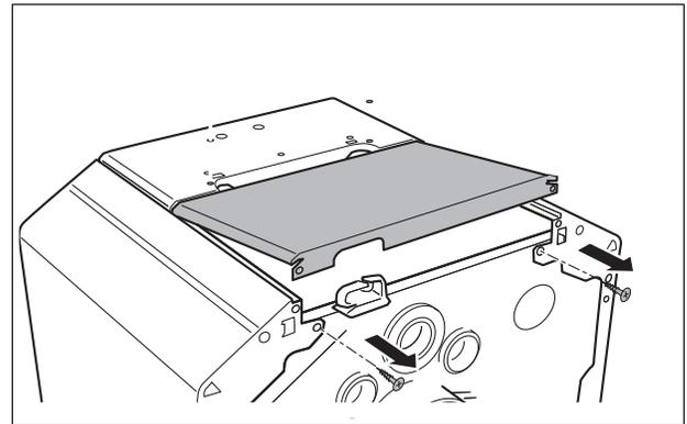
Fig. 28 Top rear cover removal
