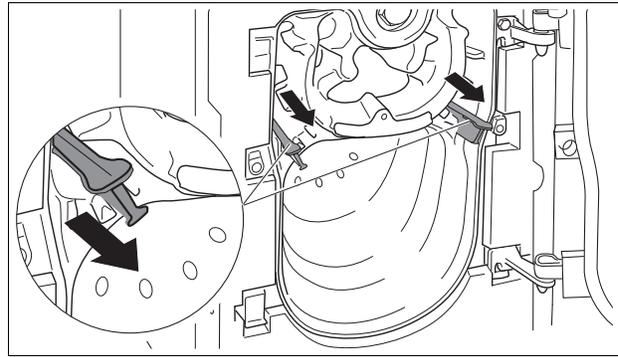
Fig.44 Removal of the flue baffles
