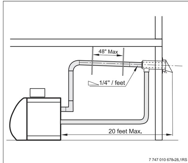
Fig. 18 Combination air intake/exhaust termination (Part No. FT-4)
