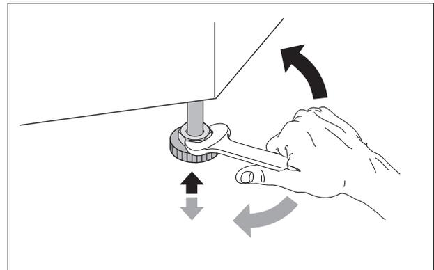
Fig. 11 Leveling the boiler
