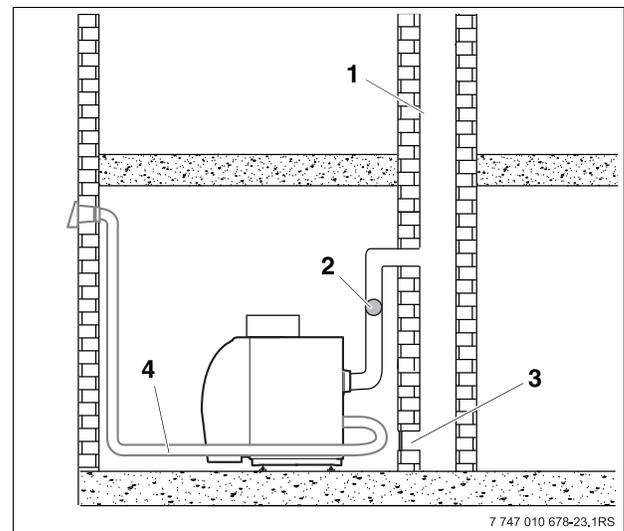
Fig. 12 Masonry chimney installation
