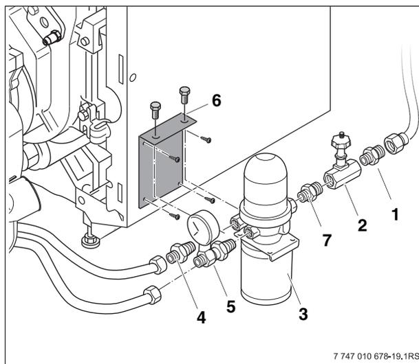
Fig. 27 Field installation of Tigerloop oil filter
