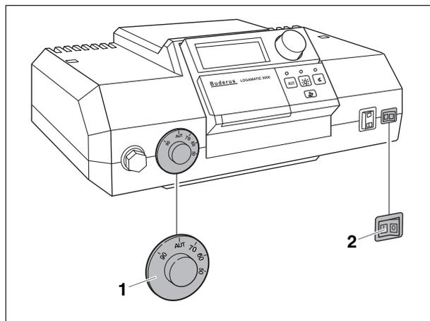
Fig.41 Switching control panel (Logamatic 2000 series controls)
