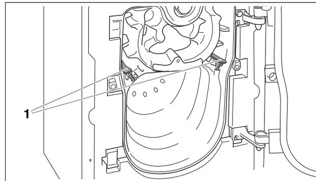
Fig.39 Opening the burner door
