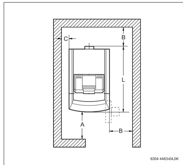
Fig. 7 Clearance dimensions for G125 boilers
