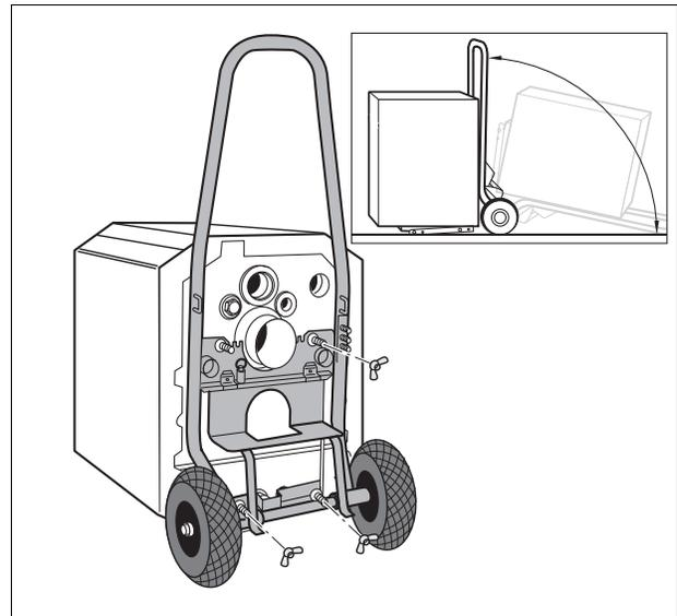
Fig. 6 Moving the boiler with a Buderus cart
