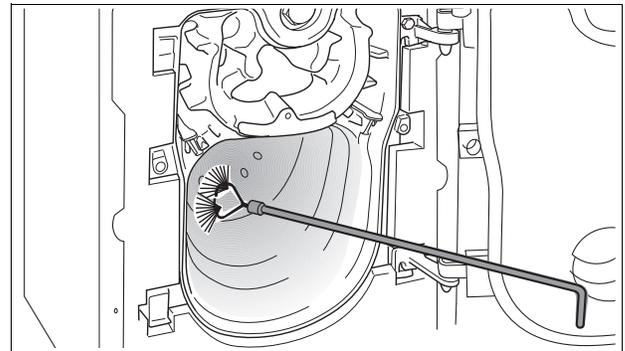
Fig. 52 Brushing out the combustion chamber
