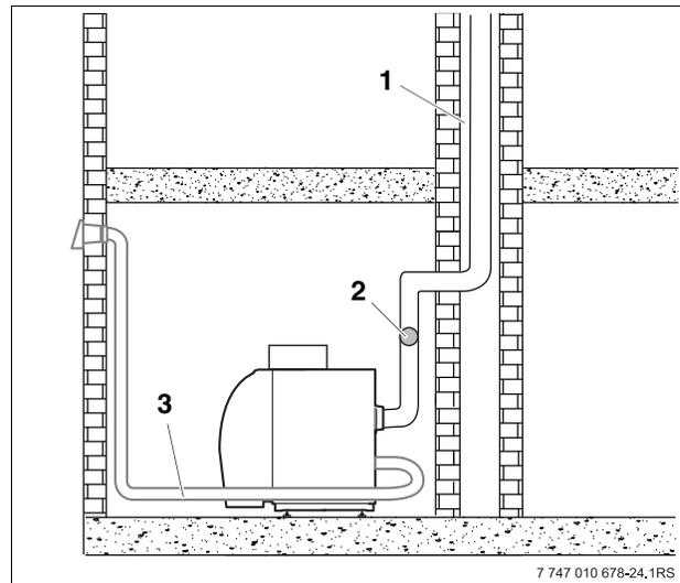
Fig. 13 5" Chimney liner installation
