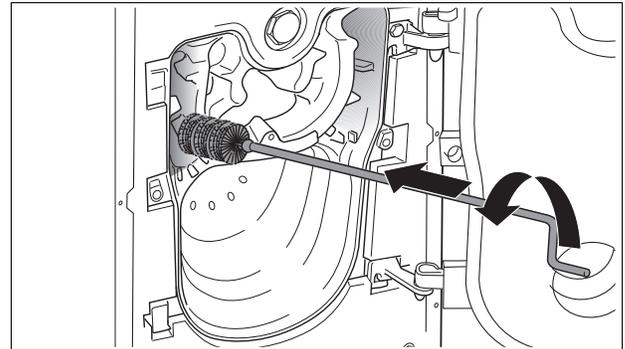
Fig. 51 Brushing out of flue passages
