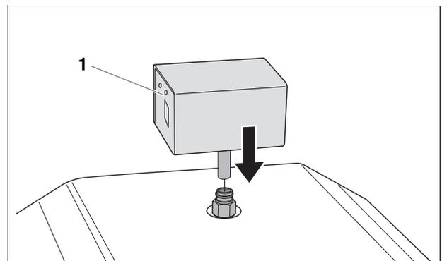
Fig. 29 Installation of Honeywell aquastat
