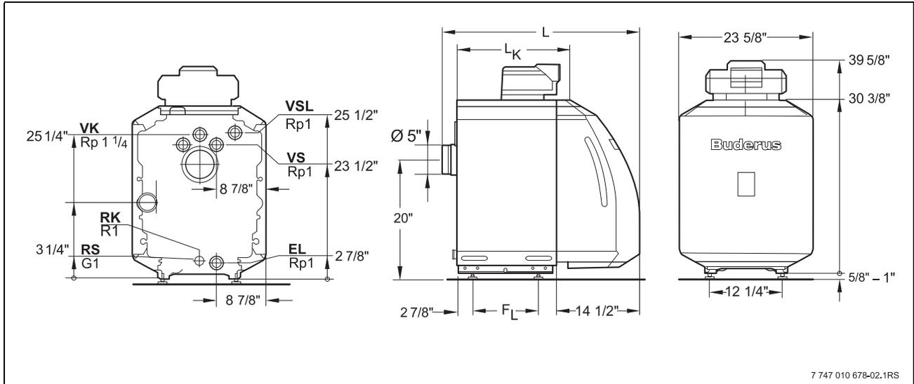
Fig. 2 Dimensions and connections (measurements in inches)
