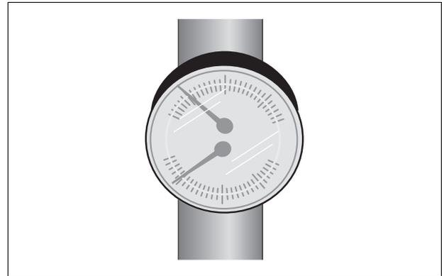
Fig. 54 Pressure/temperature gauge to display system pressure and supply temperature
