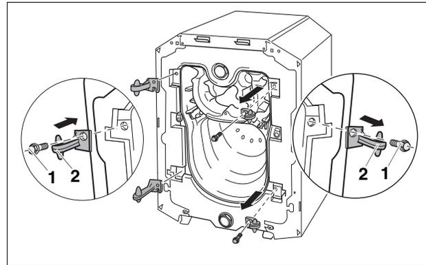
Fig. 8 Reversing burner door (boiler block)
