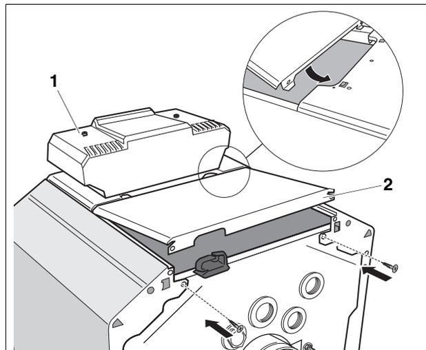
Fig. 37 Installation of rear top cover
