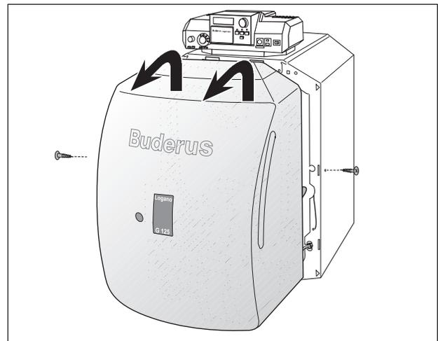
Fig. 3 Removing the front cover
