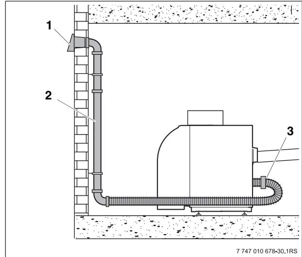
Fig. 20 Combustion air supply system
