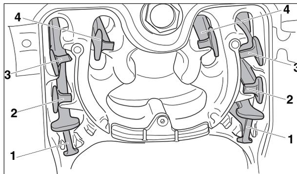
Fig.40 Blue baffle plates for fresh air operation
