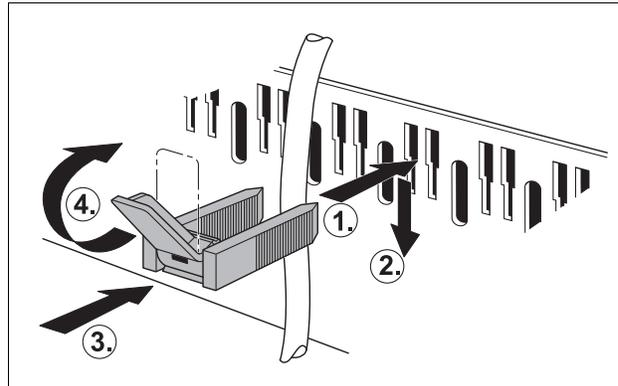
Fig. 36 Secure wiring with cable clips
