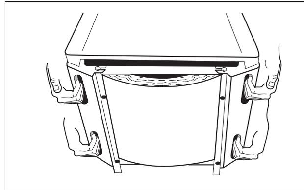
Fig. 5 Lifting and carrying the boiler
