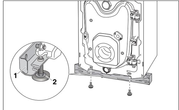
Fig. 10 Installation of boiler feet
