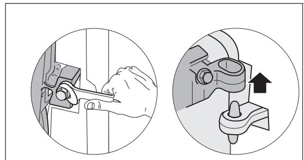
Fig. 4 Removal of burner door
