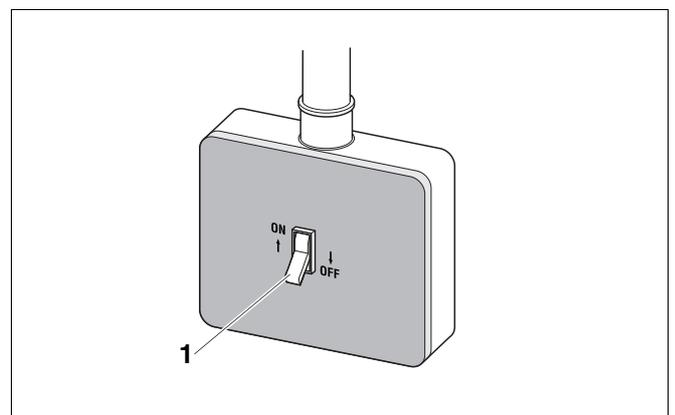
Fig. 37 Switching on heating system (with aquastat)
