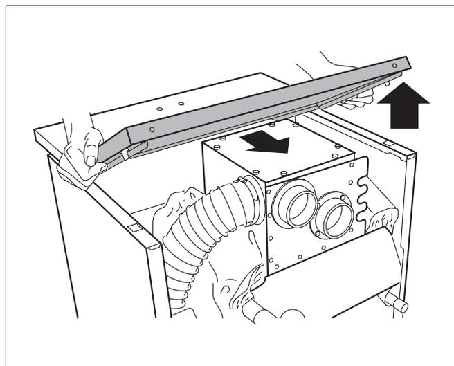
Fig. 12 Removing boiler jacket
