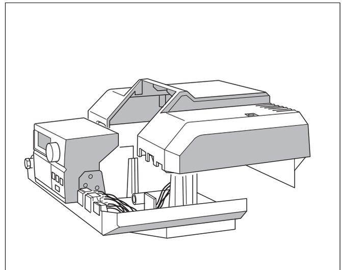
Fig. 18 Positioning terminal cover
