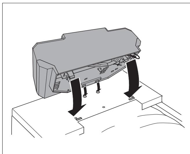
Fig. 13 Removing terminal cover
