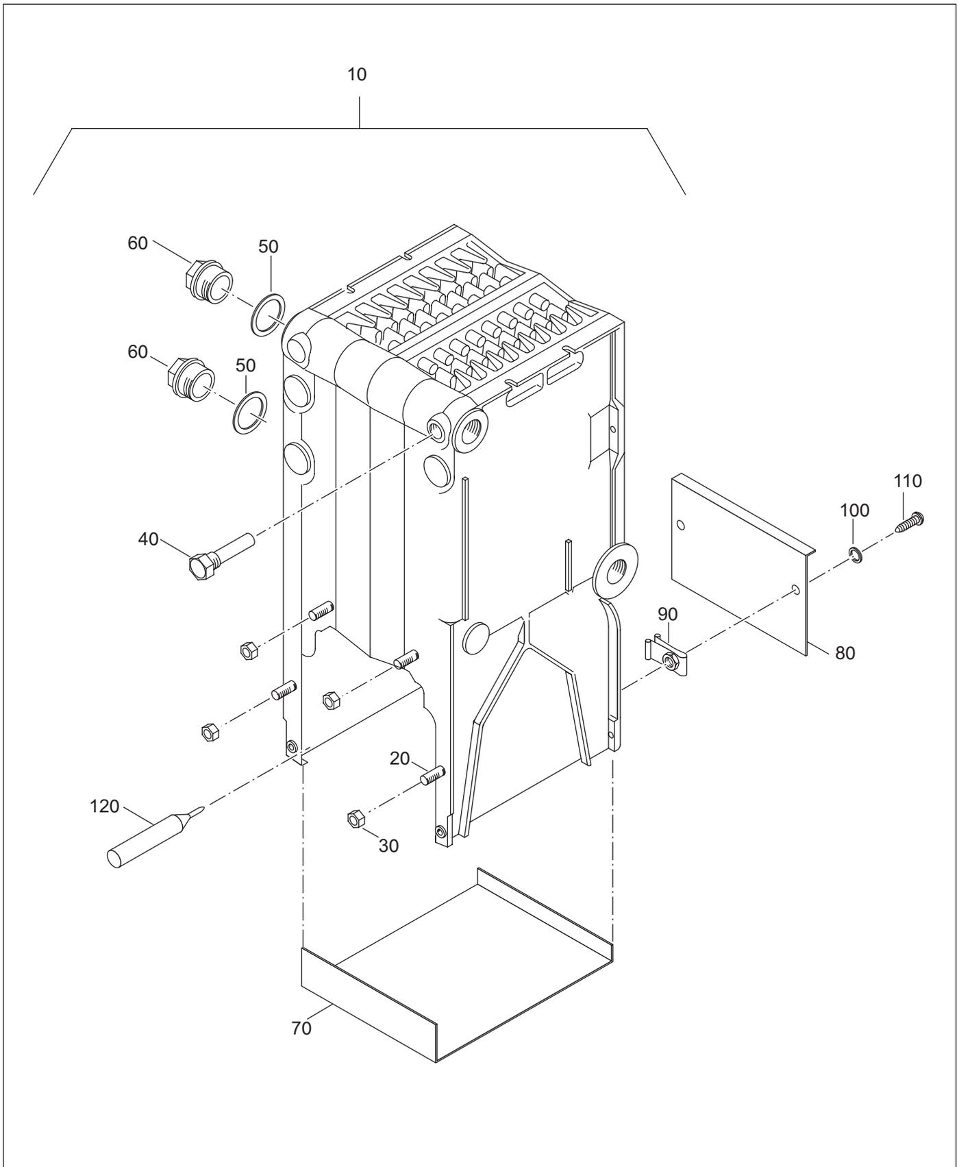
Fig. 56 Boiler block
