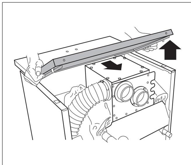
Fig. 51 Removing rear boiler jacket
