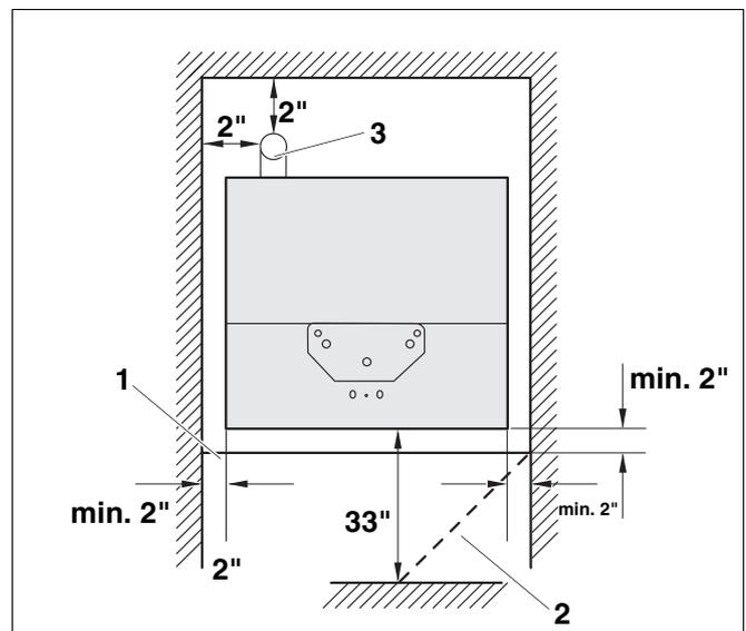
Fig. 7 Required clearances in the boiler room
