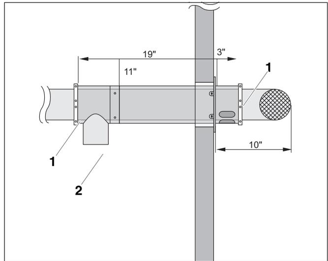
Fig. 23 Position of termination tee on the flue pipe
