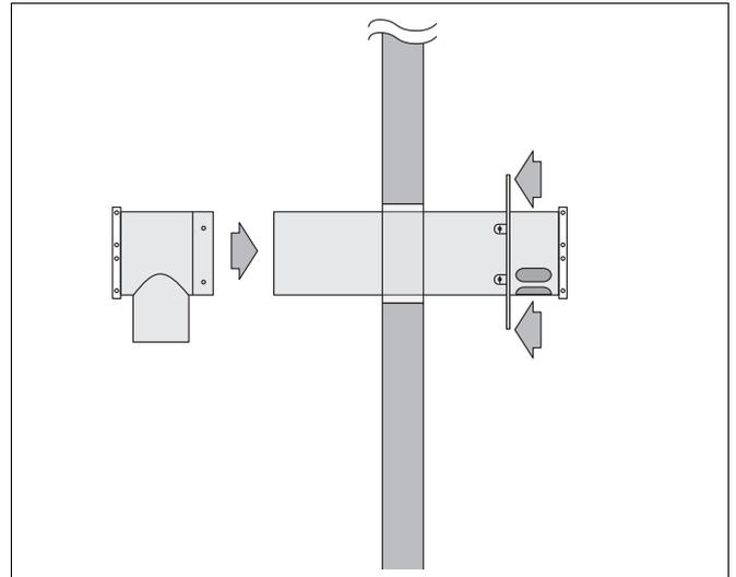
Fig. 21 Wall penetration
