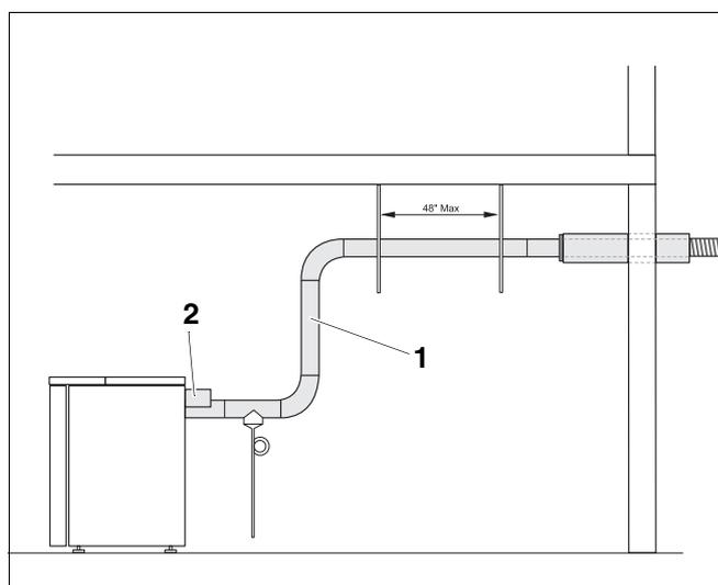
Fig. 32 Horizontal flue system using room air
