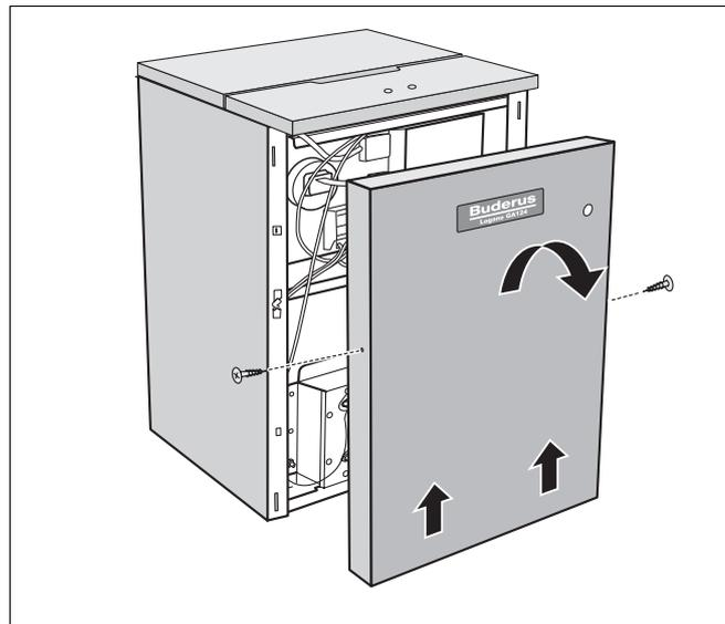
Fig. 44 Remove front panel of boiler
