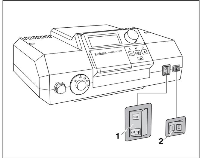
Fig. 38 Turning on heating system (with Logamatic 2107 control)
