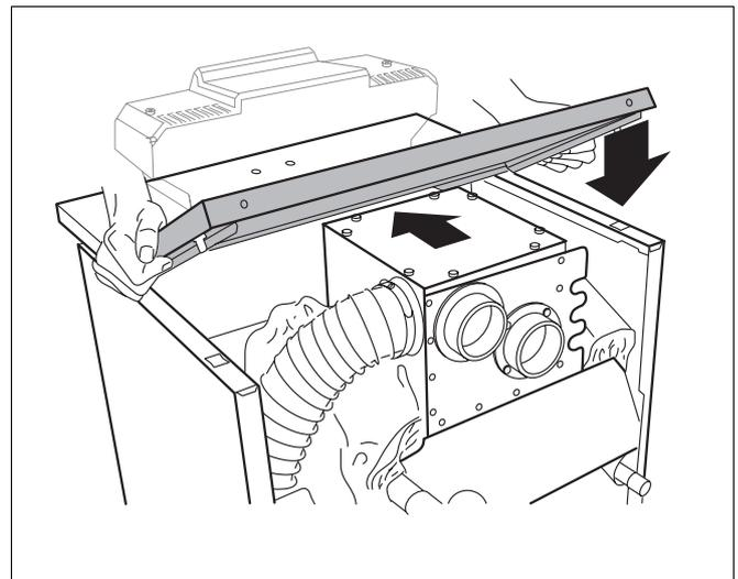
Fig. 19 Installing rear boiler cover
