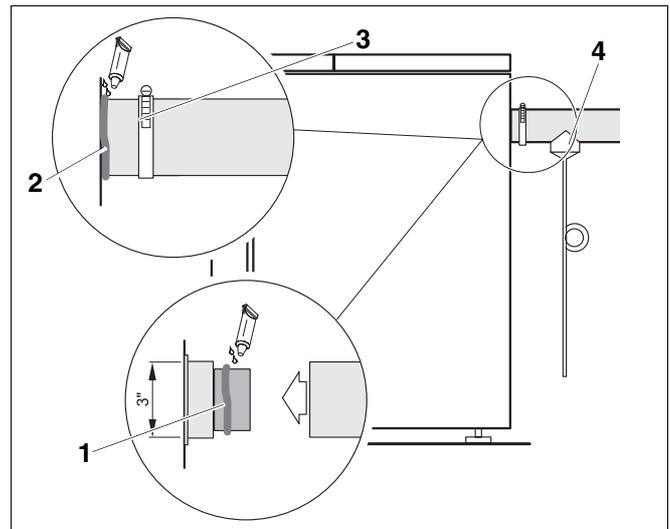
Fig. 26 Condensation trap
