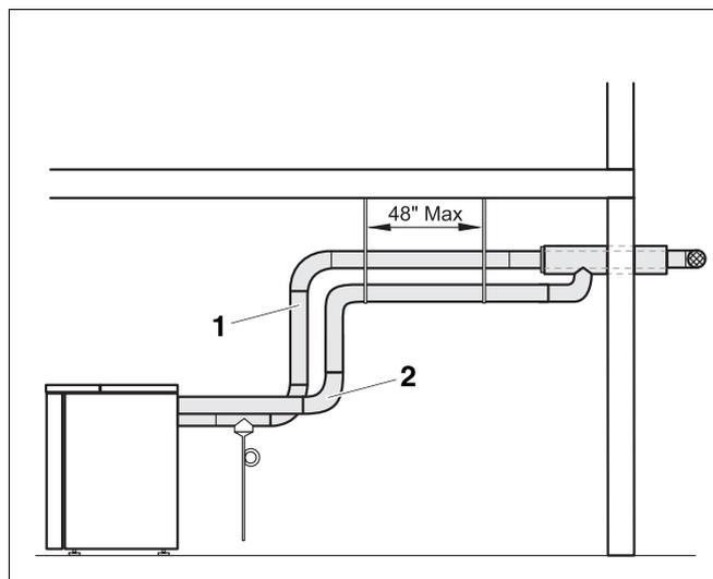
Fig. 31 Horizontal flue system independent of room air
