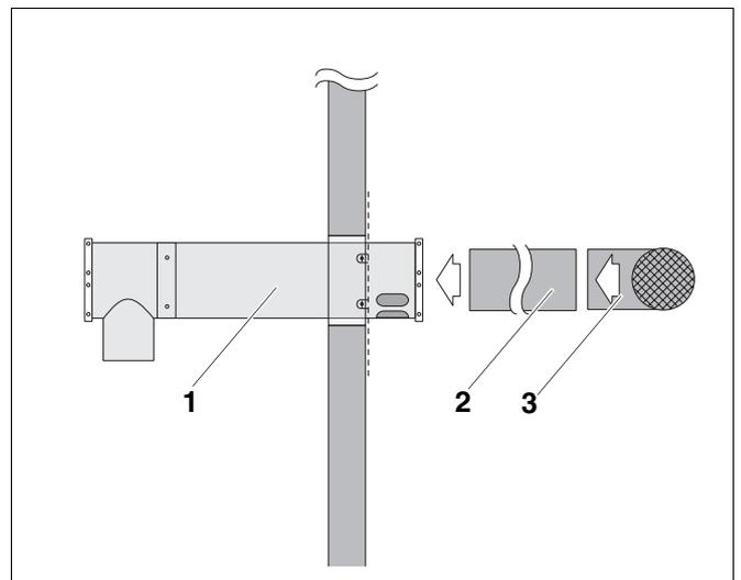
Fig. 22 Installing flue pipe
