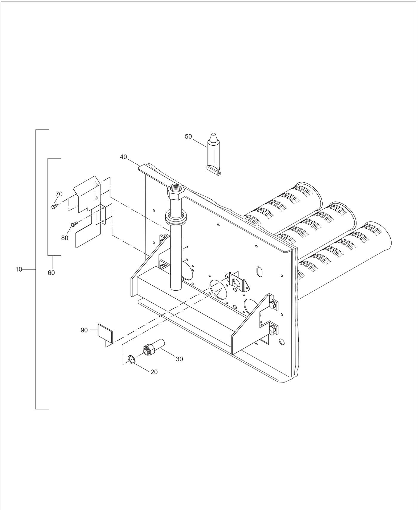
Fig. 63 Burner grate
