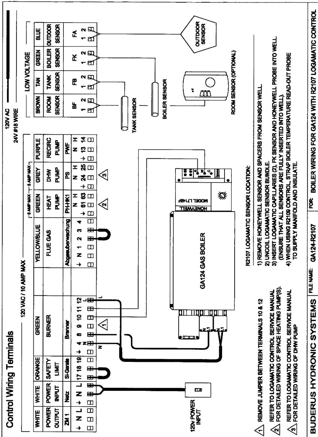
Fig. 67 Wiring diagram – GA124 with Logamatic 2107 or Logamatic 2109 control
