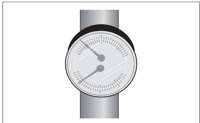
Fig. 34 Temperature/pressure gauge
