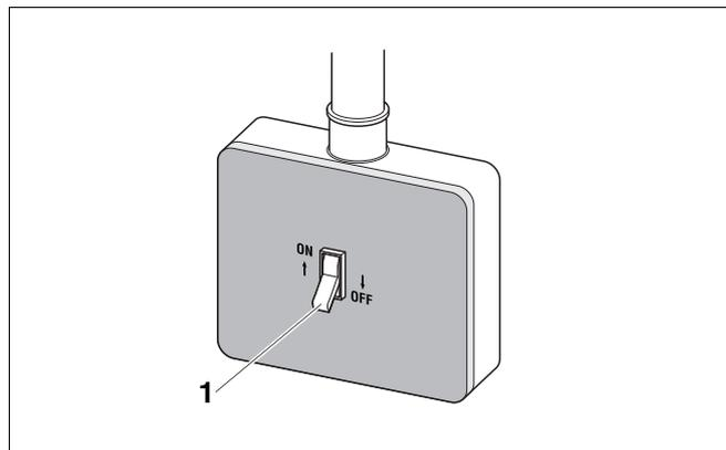
Fig. 46 Shutting down heating system (with aquastat)
