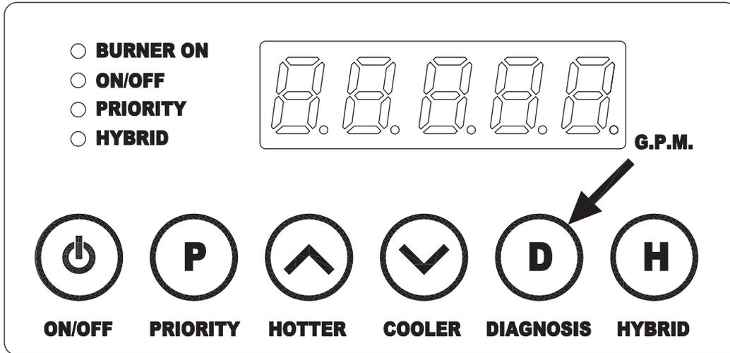
Press the "D" button when the unit is in standby mode (burner off):
