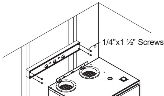
3. Hang the unit on the mounted wall bracket and secure bottom of the unit to the wall with included wall anchors and wall screws.
