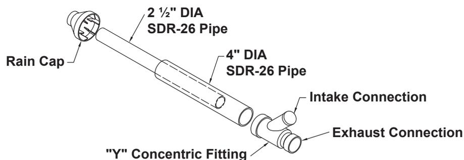
Note! When installing Horizontally, It's recommended to position the intake connection of the concentric kit to face upward to prevent rainfall/water accumulation flow through the intake pipe into the unit.
