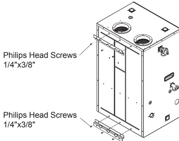
2. Select a location on the wall to mount the unit. The included wall bracket has been pre-drilled for easy installation on standard stud walls. If the framing is not standard or installing on an uneven surface, fasten 3/4" plywood to the stud wall and then attach the wall bracket.
