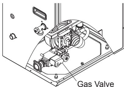
3. Loosen nut connecting gas tube to gas valve.
