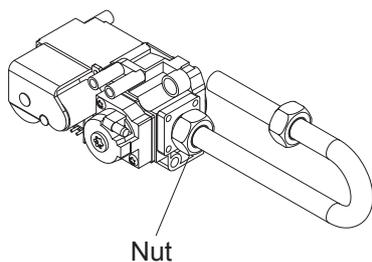
4. Insert LP orifice into the nozzle, retighten gas tube and make sure no gas leak.
