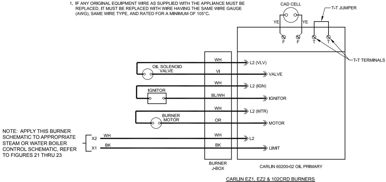
**Figure 25: Schematic Wiring Diagrams For All Burner Options w/Variou Oil Primary Controls**
