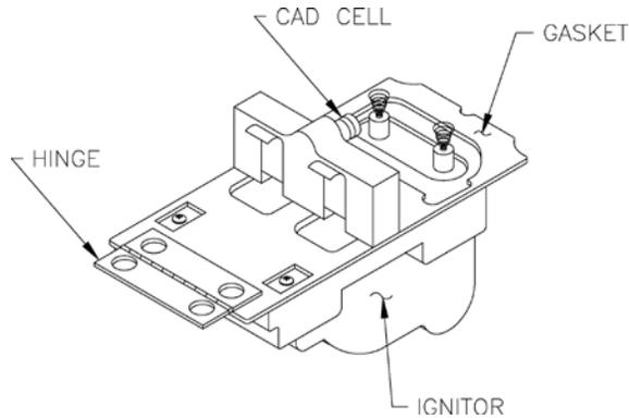
Figure 28: Cad Cell Location
