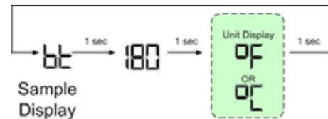
Please note that in operating mode to hold the display on the value the user can press and hold either the Up ↑ or Down ↓ keys and the value will be continuously shown. This may be helpful in watching a value "live".
