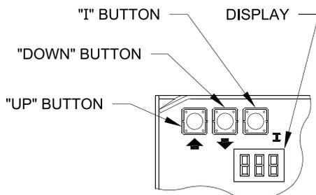
**Figure 31: Boiler Control Key Function & Orientation**
