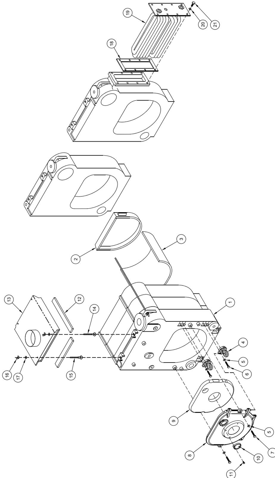
Bare Boiler Assembly (Exploded View)
