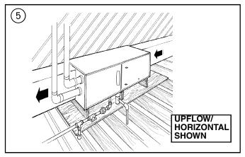
The furnace may be placed horizontally in a crawl space on a pad or other noncombustible material which will raise the unit for sufficient protection from moisture. The furnace must be supported at both ends and the middle when installed horizontally.
