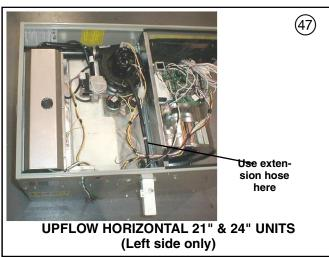
next to the secondary recuperated cell. Remove the larger drain line (from the secondary cell) and trim to fit between the secondary cell and the new trap location. On upflow units, plug the hole in the blower deck where the tube went through.
