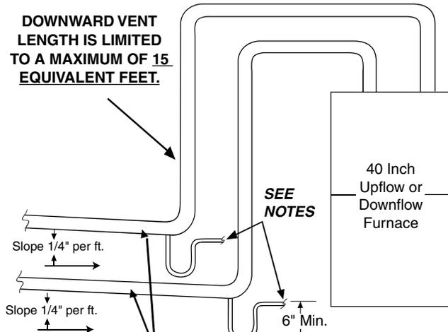
All horizontal pipes must be supported at a maximum of 3 foot intervals
