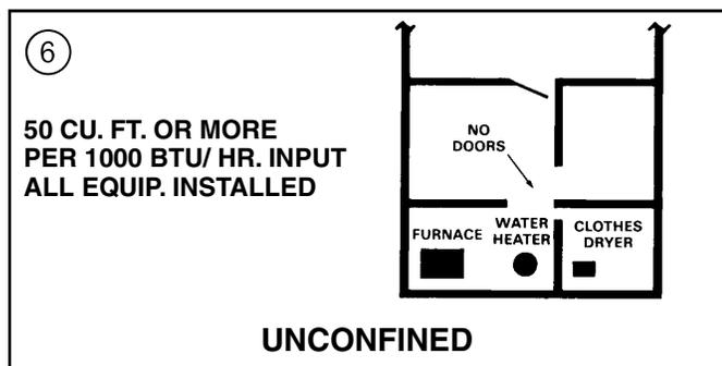
Provisions for combustion and ventilation air shall be made in accordance with latest edition of Section 5.3, Air for Combustion and Ventilation, of the National Fuel Gas Code, ANSI Z223.1 — CAN/ CGA B149.1 or applicable provisions of the local building codes. Special conditions created by mechanical exhausting of air and fireplaces must be considered to avoid unsatisfactory furnace operation.
