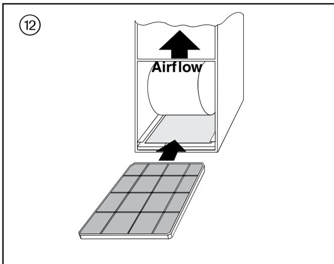
**NOTE:** The narrow 14.5" width furnace cabinet prevents use of the filter rack for right side return. Pre-drill clearance holes and then attach filter clips with the screws provided. The filter clip with the leaf spring mounts in the rear of the cabinet
