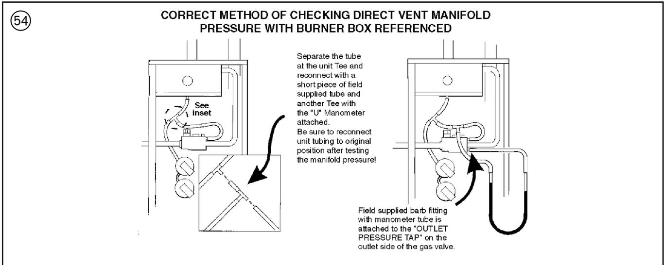
9. Using a leak detection solution or soap suds, check for leaks at the pressure outlet boss and pressure tap test screw.
