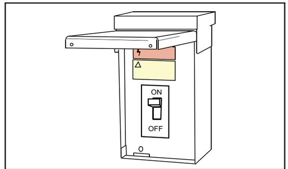
**STEP 4** - Wait one (1) hour before starting the unit if compressor crankcase heater accessory is used and the Outdoor Ambient is below 70°F.
