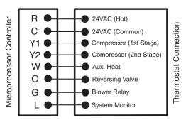
Figure 15b: Thermostat Wiring (Communicating Style Signals)
