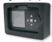
setup, and system configuration capabilities to the Aurora family of controls. An AID Tool is recommended, although not required, for ECM airflow settings. The AID Tool simply plugs into the exterior of the cabinet in the AID Tool port.
