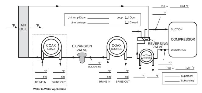
Heat of Extraction/Rejection = gpm x 500 (485 for water/antifreeze) x  $\Delta T$
