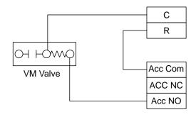
**NOTE:** SW2-4 should be "ON" and SW2-5 should be "OFF" when using a slow opening (VM) water valve.
