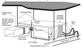
the position shown in Figure 3. The unit should be pitched approximately 1/4-inch towards the drain in both directions to facilitate the removal of condensate. Use only the bolts provided in the kit to attach hanger brackets. The use of longer bolts could damage internal parts.
