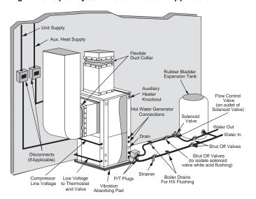
Figure 9b: Open Loop Solenoid Valve Connection Option Typical slow operating external 24V water solenoid valve (type VM) wiring and one (1) quick operating valve.
