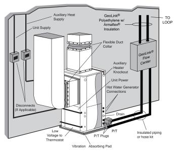
**NOTE:** Additional information can be found in Flow Center installation manual and Flush Cart manual.
