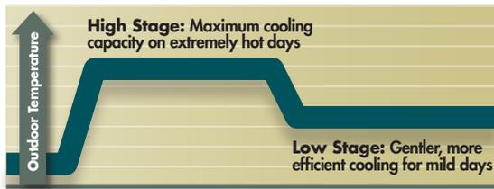
With its two-stage design, the 4SCU18LS makes the distinction between mild and extremely hot days, using only the energy necessary to keep you comfortable.
