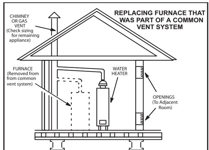
If this gas furnace replaces a furnace which was commonly vented with another gas appliance, the size of the existing vent pipe for that gas appliance must be checked. Without the heat of the original furnace flue products, the existing vent pipe is probably oversized for the single water heater or other appliance. The vent should be checked for proper draw with the remaining appliance.
