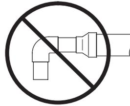
DO NOT transition from smaller to larger pipe size in horizontal runs of exhaust pipe.
