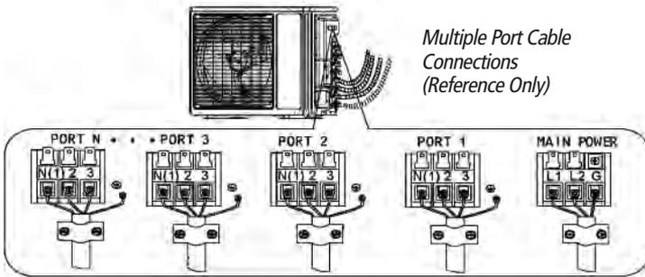
**NOTE:** Crossing interconnecting wires will cause system malfunction and possible damage.
