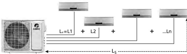
The maximum equivalent pipe length from the outdoor to the farthest indoor units (Ls) must be less than:
