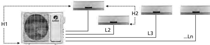
The maximum elevation (H1) from the bottom of the outdoor unit to the bottom of the highest mounted indoor units must be less than:
