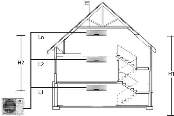
Measure and record the piping length (L1,L2, L3...Ln) from the outdoor unit to each indoor unit.
