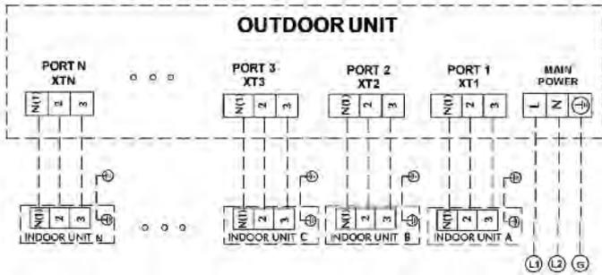
Multiple Port Wiring Diagram
