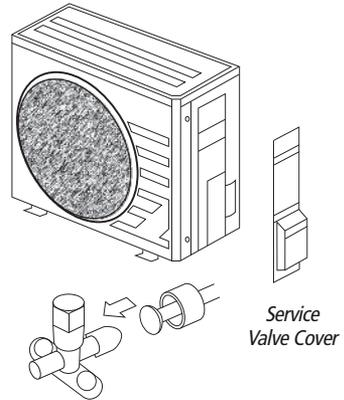
**NOTE:** Use proper techniques to cut and re-flare refrigerant pipes, if required. An R410A Flaring Tool is required for re-flaring refrigerant pipes.
