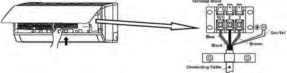
3. Connect wiring to indoor unit per connection diagram.
