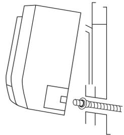
4. Open front cover of indoor unit and remove field wiring terminal block cover. Route the interconnecting wires to terminal block in control box.
