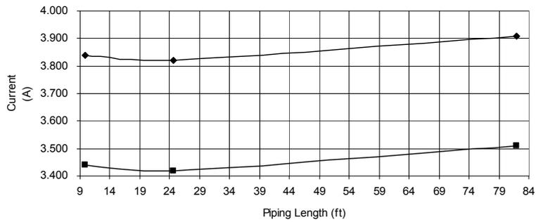
• **Piping Length Characteristic Cooling**
