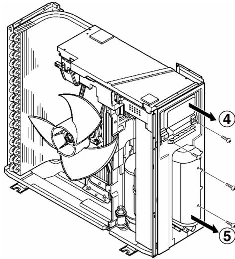
**16.1.3 Removing the Control P.C. Board**
