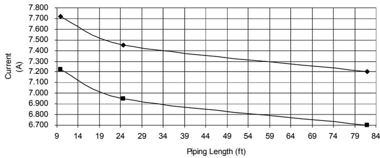
● **Piping Length Characteristic Heating**
