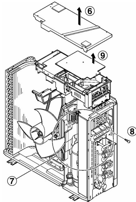
**16.1.4 Removing the Propeller Fan and Fan Motor**
