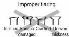
When properly flared, the internal surface of the flare will evenly shine and be of even thickness. Since the flare part comes into contact with the connections, carefully check the flare finish.
