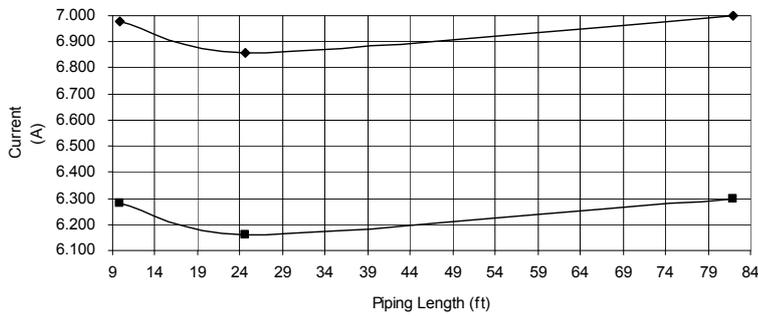
• **Piping Length Characteristic Cooling**
