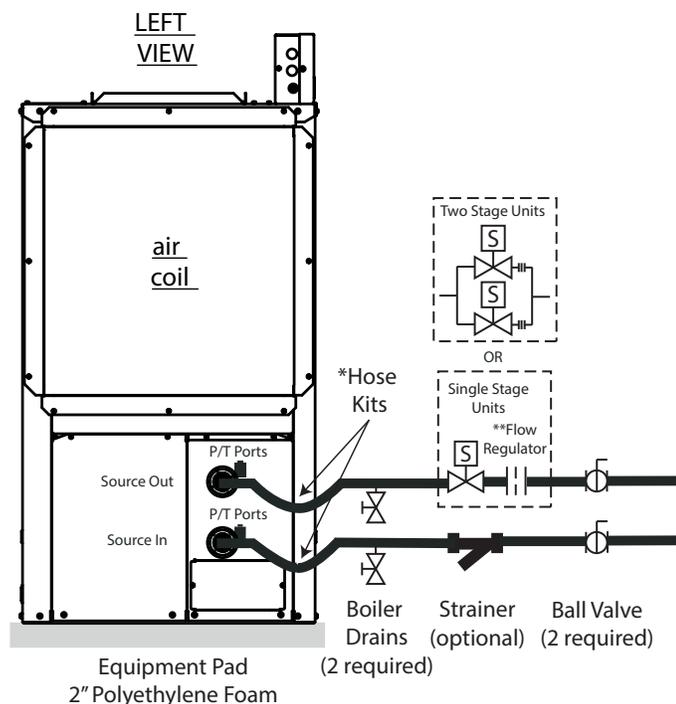
\*Hose kit is used for piping isolation, and includes fittings for P/T ports.
