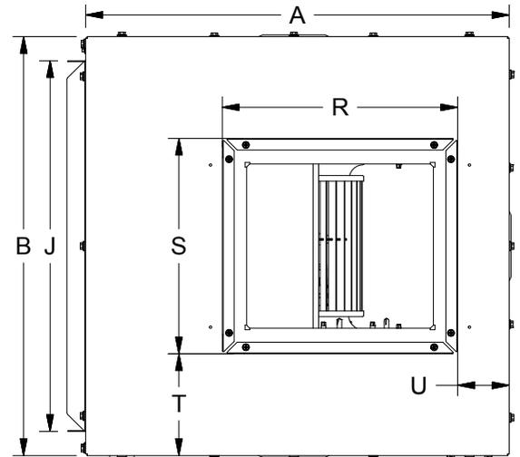
**Enertech Recommends A Minimum of 2 to 2 1/2 Feet of Service Area Clearance For Installation And Maintenance.**
