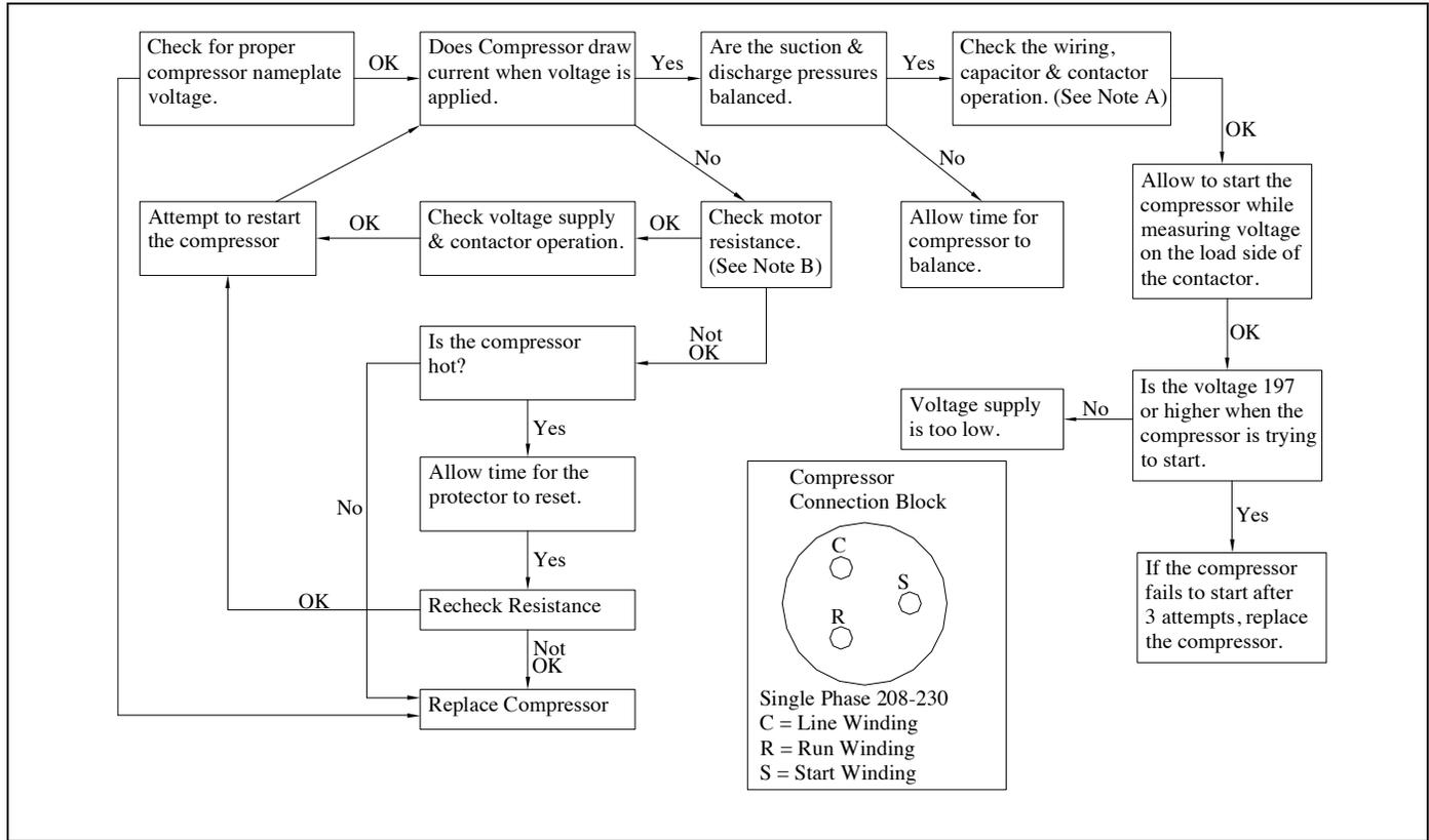
A: Check all terminals, wires & connections for loose or burned wires and connections. Check contactor and 24 Volt coil. Check capacitor connections & check capacitor with capacitor tester.
