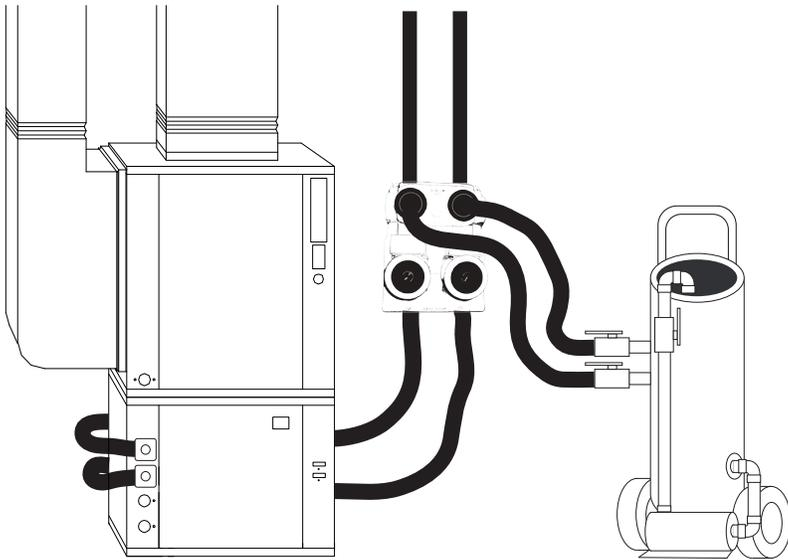
Figure 8: Flow Center 3-Way Valves
