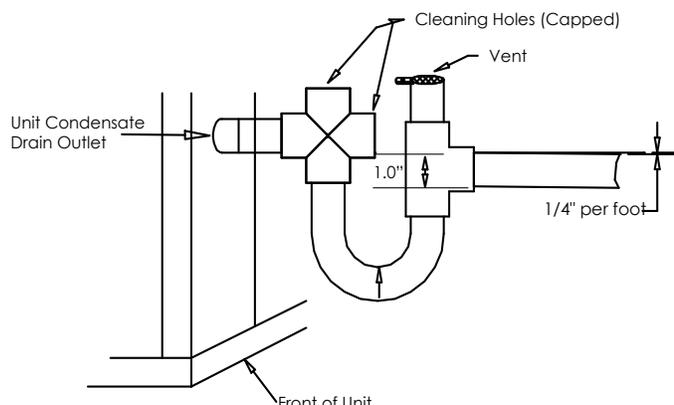
**Note:** Connect the drain through the trap to the condensation drain system in conformance to local plumbing codes.
