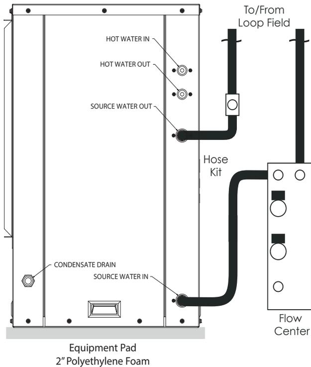
**Notes:** P/T ports should be angled away from the unit for ease of gauge reading. Drawings represent typical installation. The manufactures installation guides should be used for final installation
