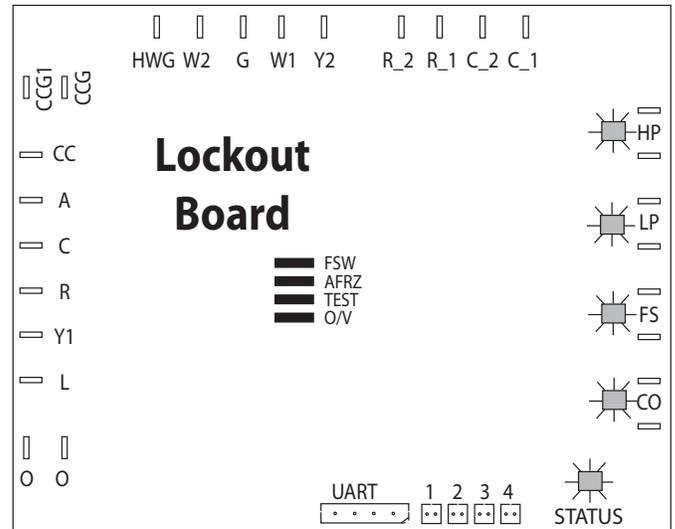
**Low Pressure-LP:** If the low pressure switch is open continuously for 30 seconds, the compressor operation will be interrupted, and the control will go into fault retry mode. At startup, the low pressure switch is not monitored for 30 seconds to avoid nuisance faults. (If the low pressure switch is open before startup then the unit will not start upon receiving an Y1 call and will lock out instead.)
