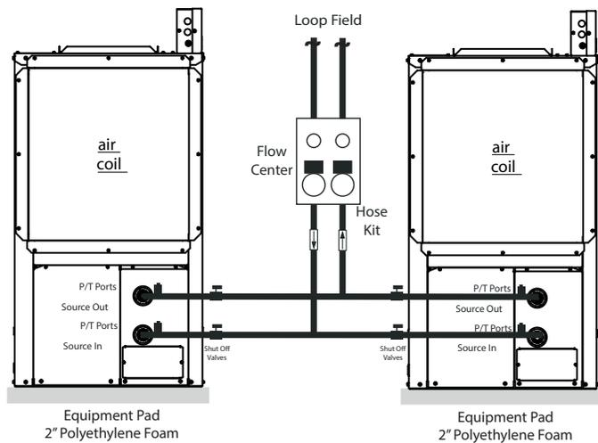
Figure 16: APSMA Module Layout
