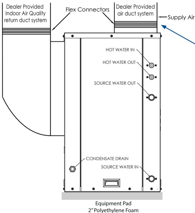
**NOTE: Maintain duct size of supply flange for at least 12" before transitioning to size of supply plenum designed for duct system.**
