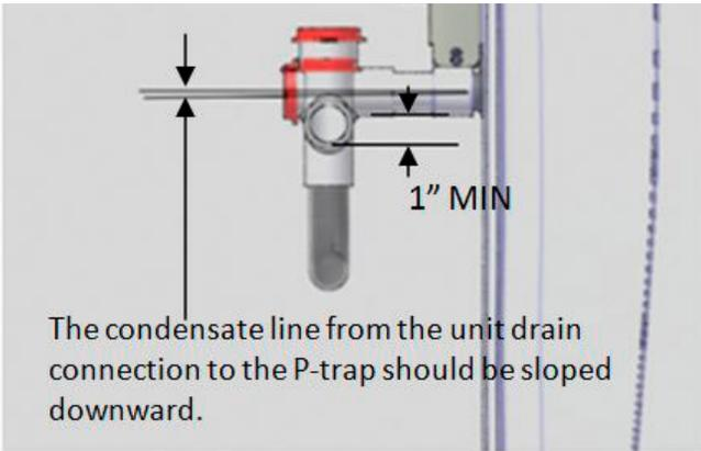
**Figure 9b: Condensation Drain Drop**
