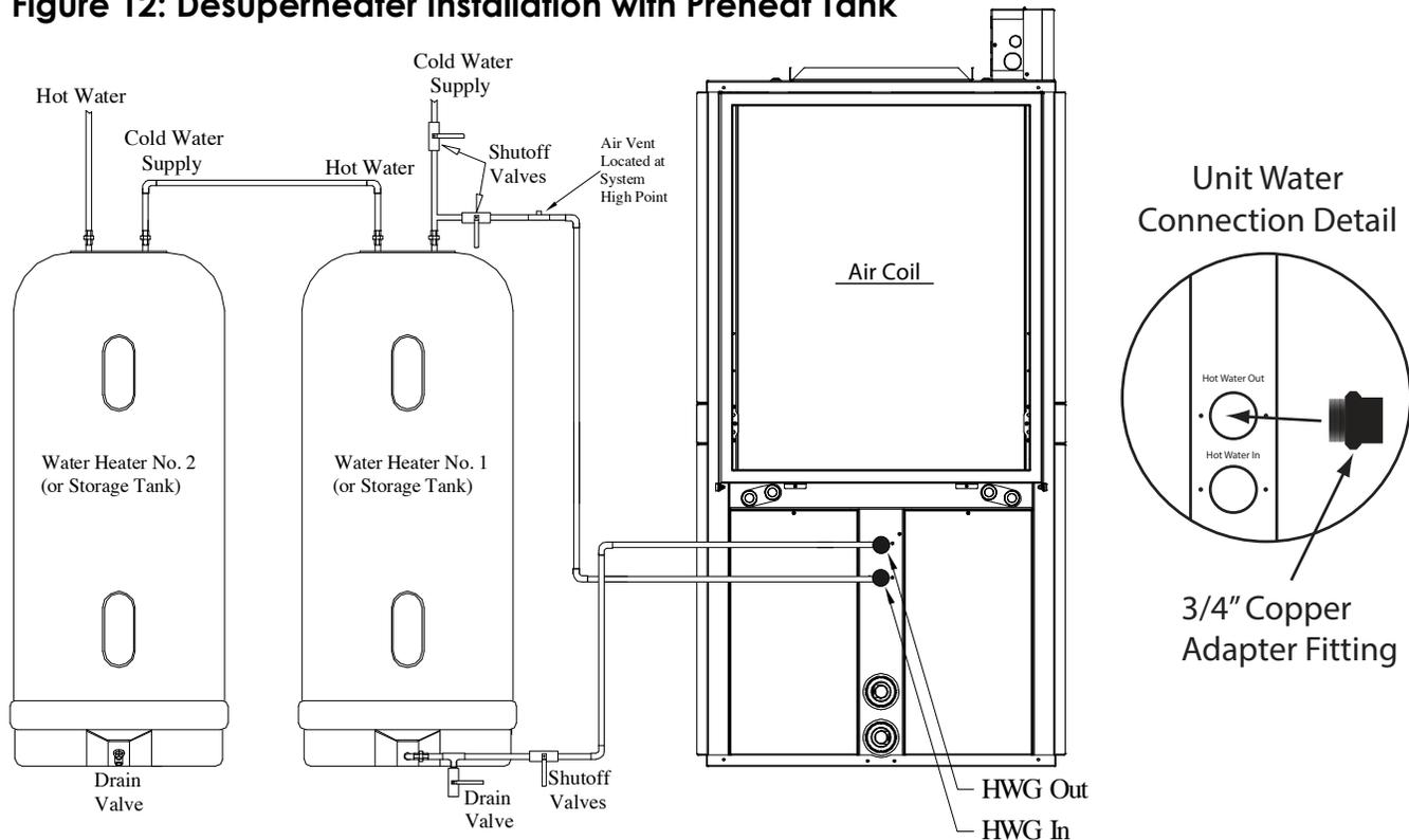
Desuperheater circuits are **NOT** to be connected to gas water heaters!
