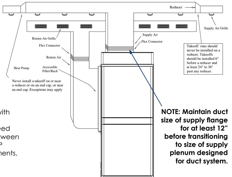
The geothermal unit comes with an ECM Motor. For maximum performance, the blower speed should be set to maintain between 350 and 450 CFM/ton. Use DIP switch for ECM motor adjustments.
