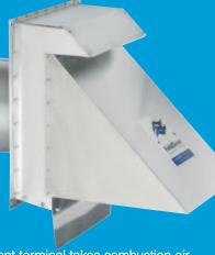
Concentric vent terminal takes combustion air in through outer ring, gets heated slightly by the exhaust air in the inner ring and insulates the exhaust from building construction.
