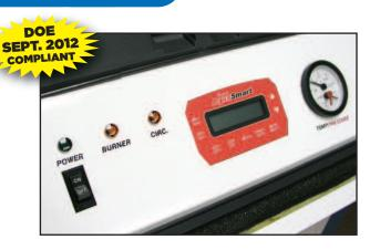
The Eutectics special control contains a Department of Energy (DOE) 2012 compliant load-matching energy saving algorithm. This feature saves fuel by dynamically changing the temperature high operating limit to the minimum temperature necessary to meet the heating demand. The qualified service technician can adjust the algorithm to align comfort and energy savings.
