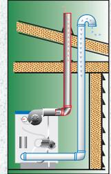
The Victory VSPH boiler operates in total isolation from household air. The combustion process is "sealed" inside the boiler, with intake air and exhaust pipes connected directly to the outdoors. Venting may be through the wall or through the roof.
