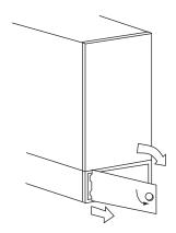
Fig. 22 - Removal of Filter Cabinet Door from Bottom
