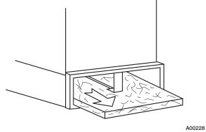
Fig. 24 - Removal of Filter from Bottom Blower Cabinet
