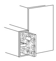
$${\tt A00227}$$  Fig. 23 - Removal of Filter from Side Blower Cabinet
