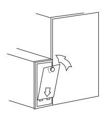
Fig. 25 - Replacement of Filter Cabinet Door to Side Blower
