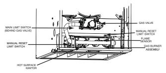
Fig. 28 - Gas Burner Assembly (Downflow)
