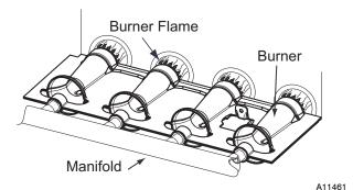
Fig. 29 - Burner Flame Adjustment
