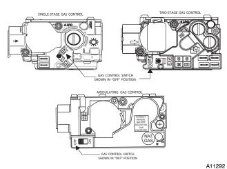
Fig. 11 - Control Switch to OFF
