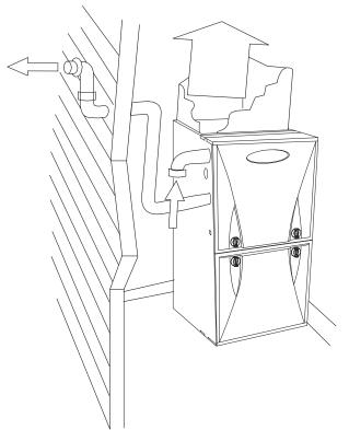
Fig. 3 - Interior Combustion - Air Pipe
