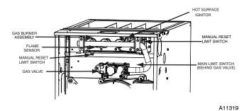
Fig. 27 - Gas Burner Assembly (Upflow)
