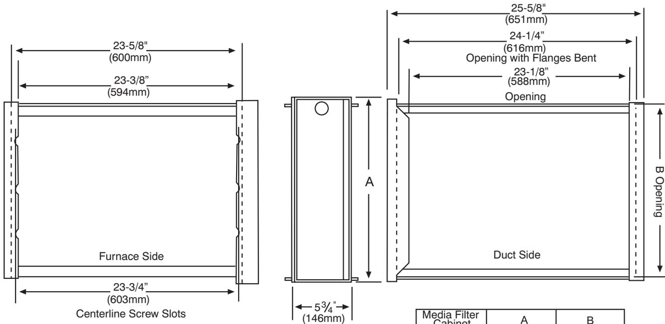
NOTE: Media cabinet is matched to the bottom opening on furnace. May also be used for side return.
