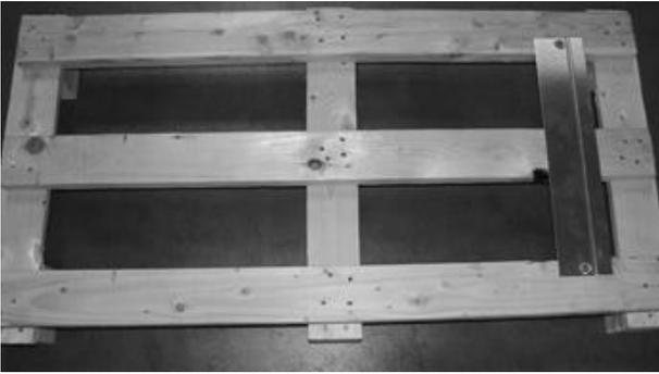
Figure 4 – Pallet with Mounting Bracket Affixed
