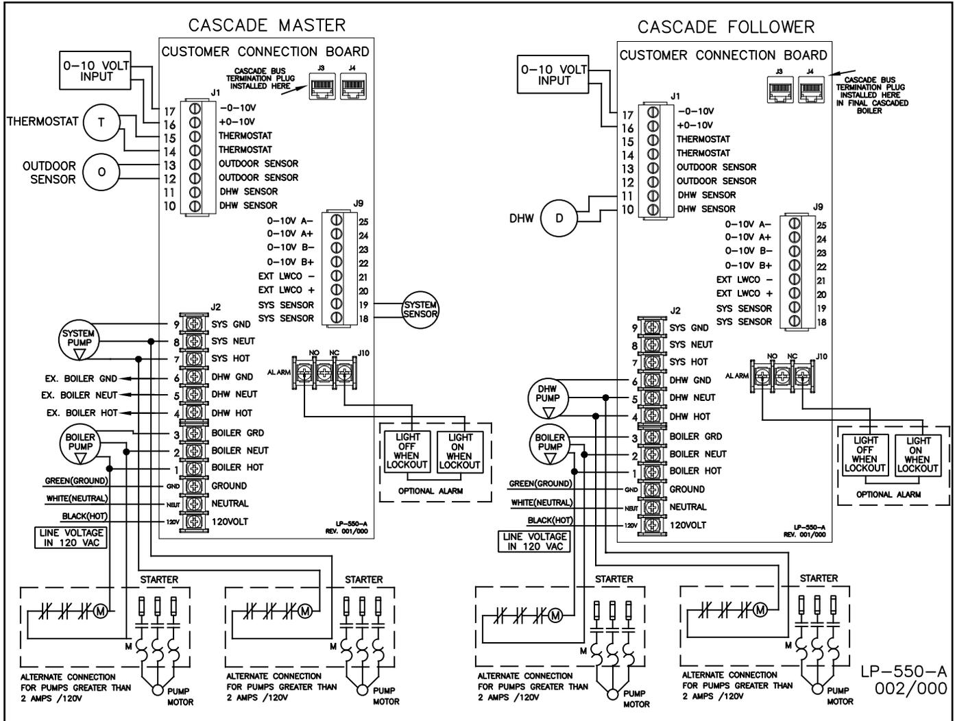
Figure 24 - Cascade Master and Follower Wiring
