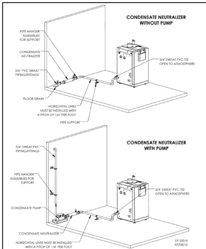
**Figure 20 - Condensate Piping**
