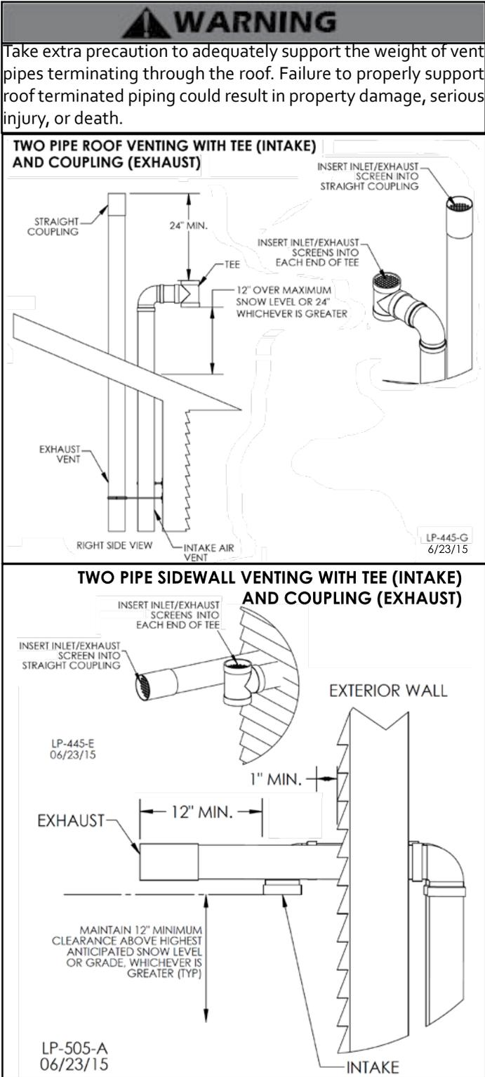
Figure 13 - Two Pipe Roof and Sidewall Venting
