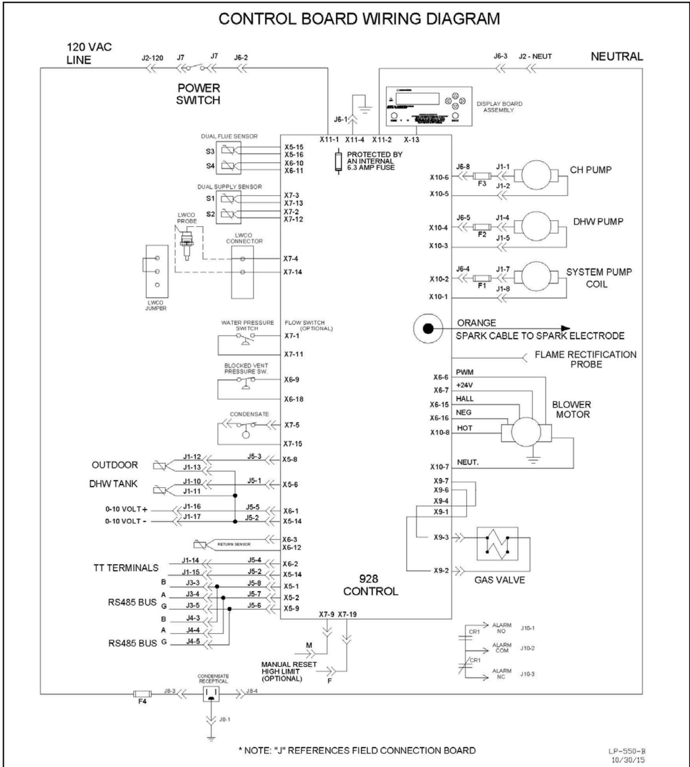
Figure 25 - Internal Connection Diagram
