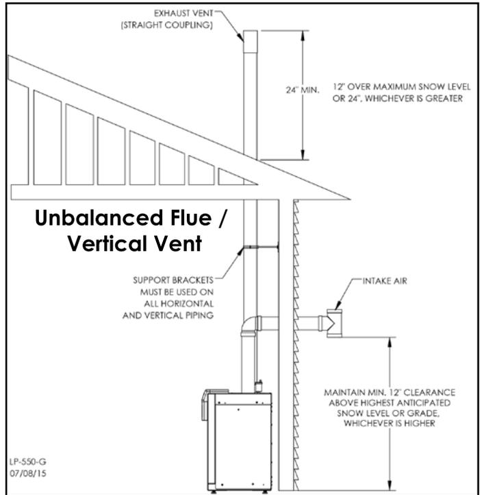
Figure 16 - Unbalanced Venting - Roof Exhaust and Sidewall Intake
