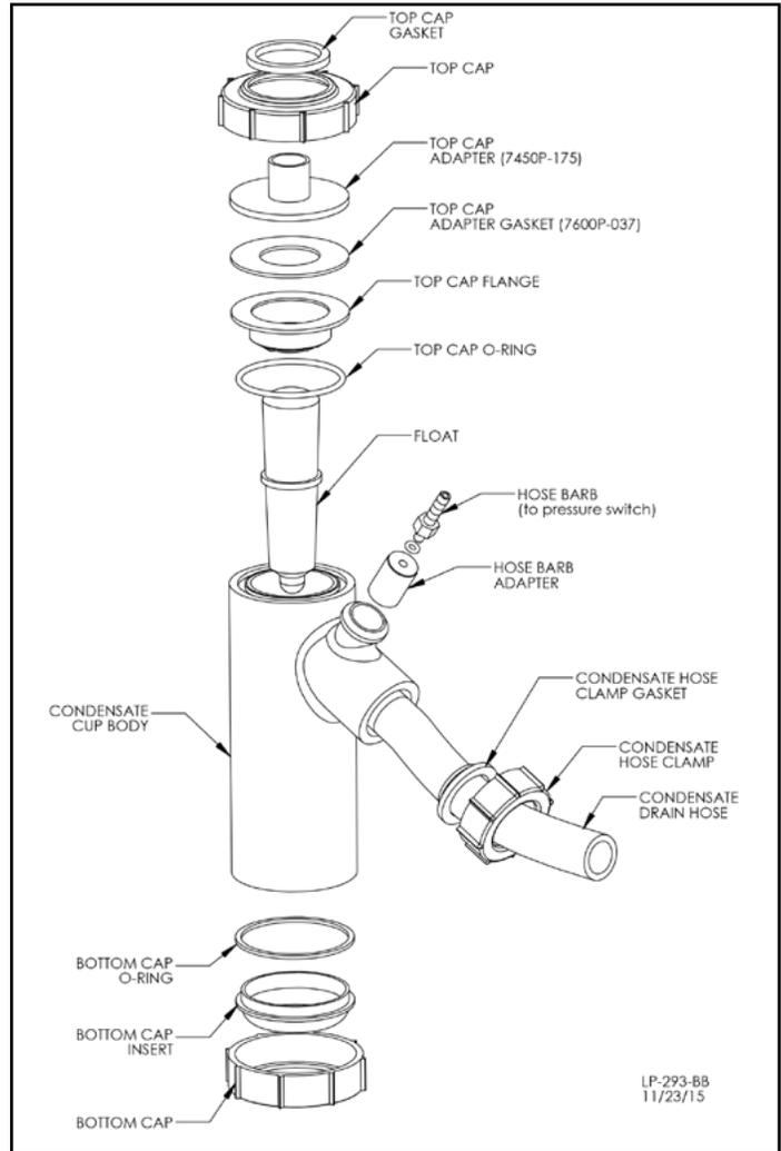
Figure 29 - Condensate Detail
