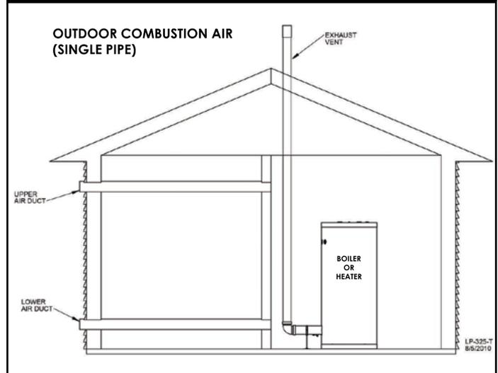
Figure 19 - Indoor and Outdoor Combustion Air - Single Pipe
