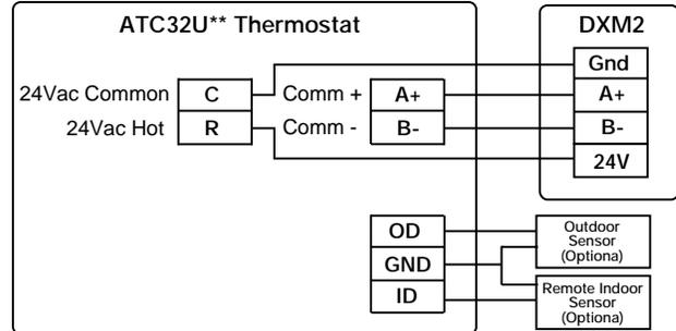
**Figure 26b: Conventional 3 Heat / 2 Cool Thermostat Connection to DXM2 Control**
