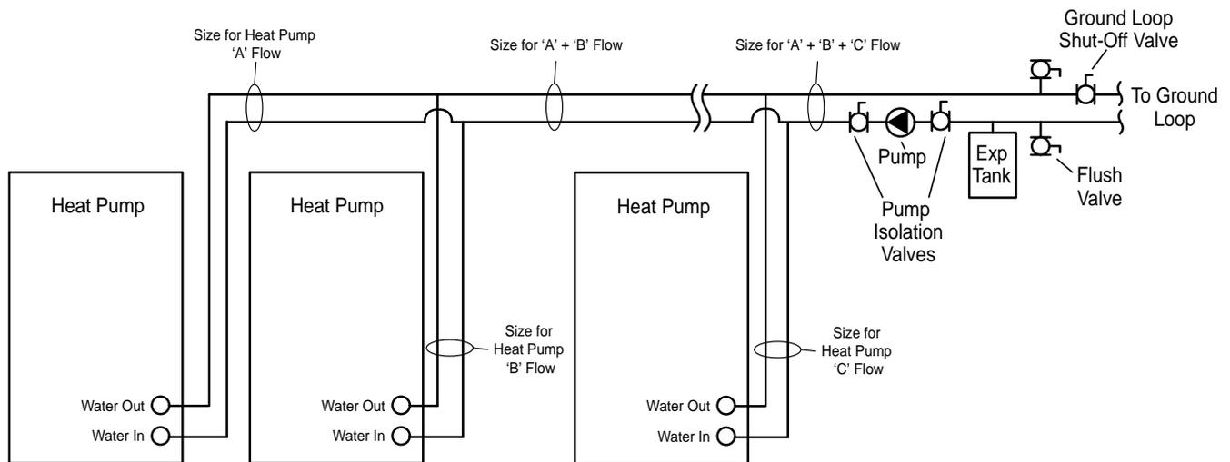
Before flushing, the installer should manually open all modulating valves as detailed in Closed Loop – External Central Pumping section of this manual. Next, flush the ground loop. The installer should close a pump isolation valve and open the ground loop shut-off valve to prevent flow through the indoor loop while flushing the ground loop.
