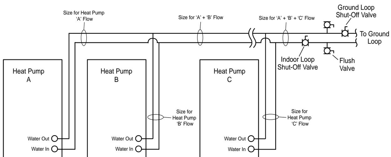
First, flush the ground loop. The installer should close the indoor loop shut-off valve (or the internal flushing valves in all units) and open the ground loop shut-off valve to prevent flow through the indoor loop while flushing the ground loop.
