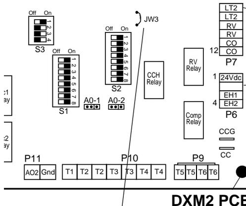
JW3-LT1 jumper should be clipped for low temperature operation
