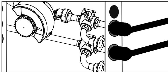
Test individual horizontal loop circuits before backfilling. Test vertical U-bends and pond loop assemblies prior to installation. Pressures of at least 100 psi [689 kPa] should be used when testing. Do not exceed the pipe pressure rating. Test entire system when all loops are assembled.
