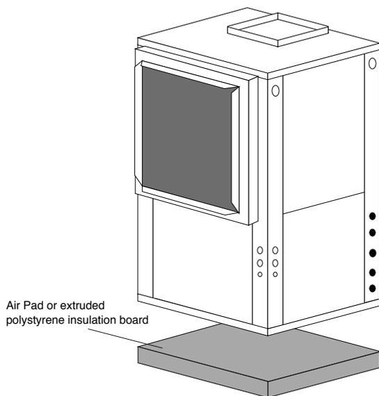
**Figure 2: Typical Vertical Unit Installation Using Ducted Return Air**
