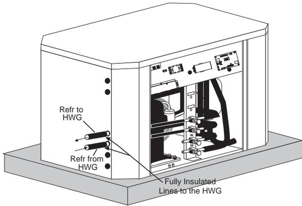
Figure 21d: HWG Service Valves
