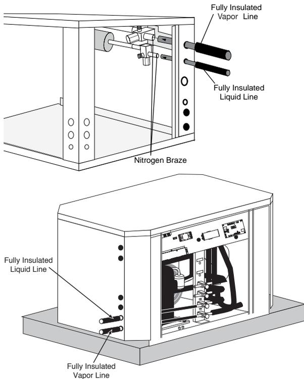
Figure 15: Air Coil Connection
