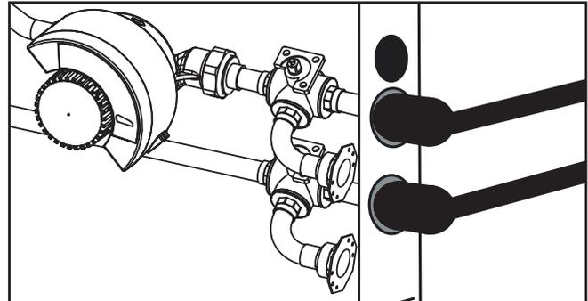
Flow rates between 2.25 and 3 gpm per ton [2.41 to 3.23 l/m per kW] of cooling capacity is recommended in these applications.
