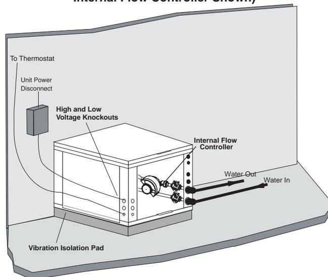
**Figure 4b: Typical Open Loop Application (with Internal Modulating Motorized Valve Shown)**
