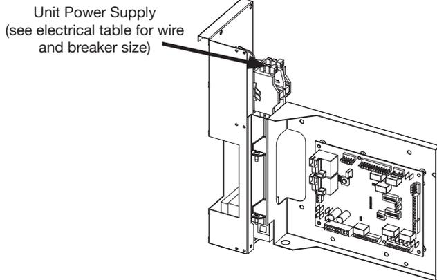
**Figure 23: Outdoor Compressor Section (TEP) Line Voltage Field Wiring**
