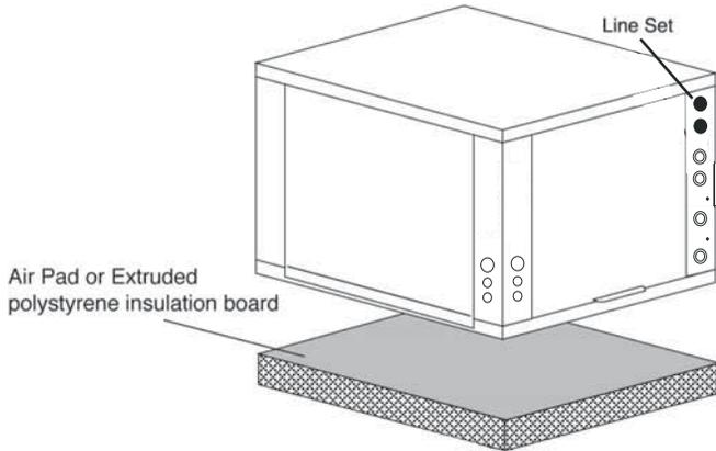
Figure 3: TEP Installation
