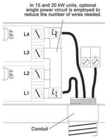
**Figure 16: Power Wiring, 4, 5, 8, and 10kW**
