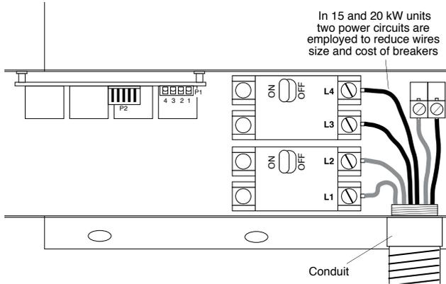
**Wiring and Setup (all models)**
