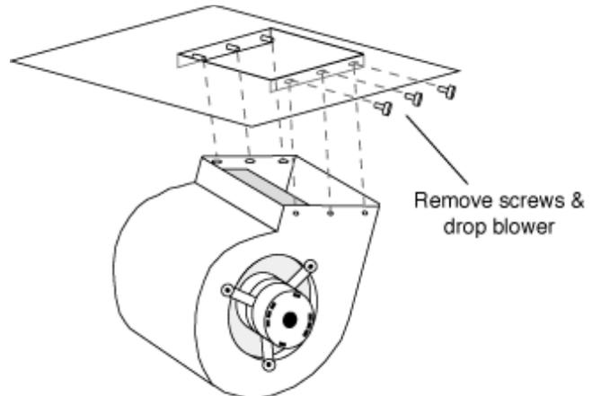
Figure 13: AG electric heat mounting and blower re-installation
