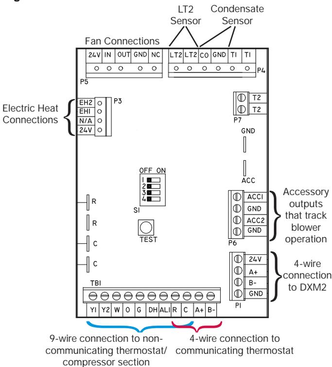
**DIP #2:** Dehumidification Mode - Provides selection of normal or Dehumidification Fan Mode. In Dehumidification Mode, the fan speed will be adjusted for Cooling. In Normal Mode, the fan speed will be normal during Cooling.
