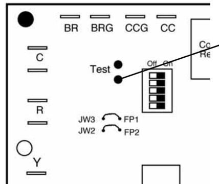
Short test pins together to enter Test Mode and speed-up timing and delays for 20 minutes.
