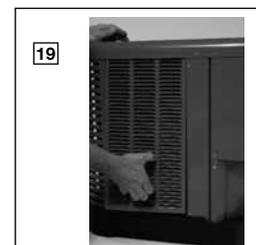
The outdoor fan motor has sleeve bearings and is inherently protected. The motor is totally enclosed for maximum protection from weather, dust and corrosion. (20) Access to the outdoor fan is made by removing four fasteners from the fan grille. The outdoor fan can be removed from the fan grille by removing 4 fasteners in the rare case outdoor fan motor fails.
