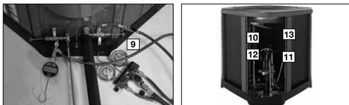
27 square-inches around the service valves allows ample room to remove service valve schrader prior to brazing, plenty of clearance for easy brazing of the suction and discharge lines to service valve outlets, easy access and hookup of low loss refrigerant gauges (9), and access to the service valve caps for opening.
