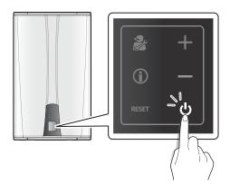
When the power is on, the temperature will appear on the front panel display.
