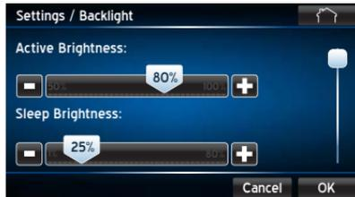
*Your brightness default settings are preset to maximize the life of your Communicating Control. Increasing the brightness levels could potentially decrease the life of the product. Brightness default settings for your Communicating Control are set: Active Mode Brightness 80% and Sleep Mode Brightness 25%.*
