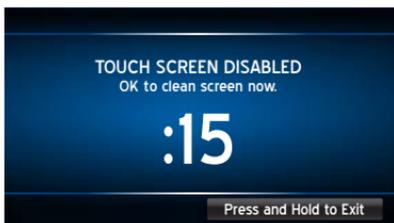
2. Press **Clean** icon to lock the screen for cleaning. The screen will remain locked for 15 seconds to allow you to clean the screen without changing any settings. After 15 seconds, normal screen operation will resume. If more time is needed for cleaning, repeat steps 1 and 2 above.
