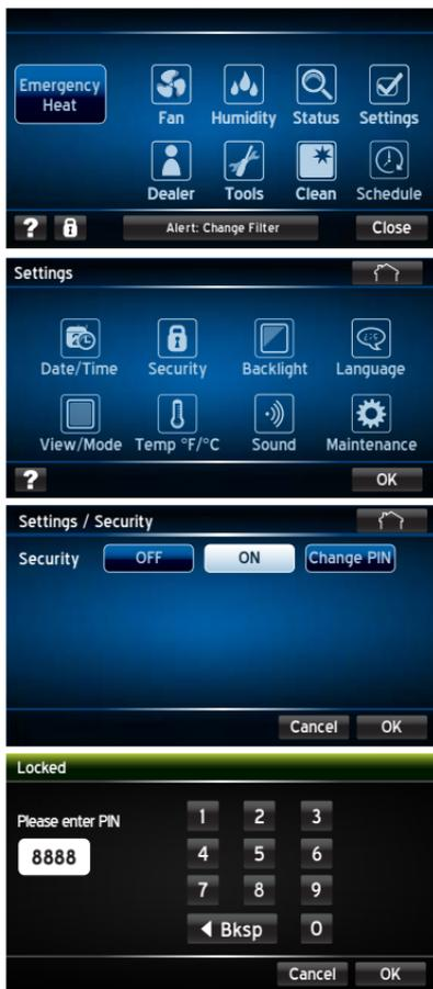
To prevent tampering with your Communicating Control, the screen can be fully locked. To activate the screen security setting, follow these steps:
