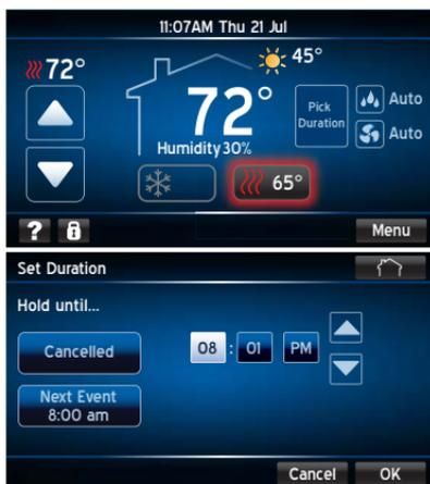
1. Press **temperature adjustment arrows** either up or down until the desired override temperature setpoint is shown.
